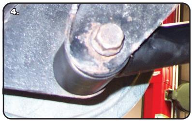
**4.** Attach to rear of the lower StrongArm to the frame using the  $\frac{1}{2}$ " x 3  $\frac{1}{2}$ " bolts, flat washers and nylok nuts supplied.
