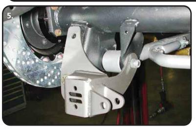
**5.** Remove the lower trailing arm mounting bolt. (Do one side at a time to keep the axle from rotating). Install the longer  $\frac{1}{2}$ " x 3  $\frac{3}{4}$ " bolt through the lower trailing arm from the outside in. Install the lower bracket over the bolt and secure with a  $\frac{1}{2}$ " Nylok nut and flat washer. Snug the Hardware, but do NOT fully tighten at this time.
