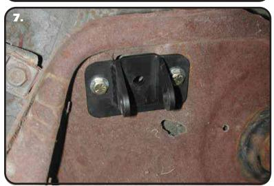
**7.** Fasten the new upper shock bracket into the factory shock location using the 5/16" x 1" bolts, flat washers and Nylok nuts supplied. Torque to 17 ftlbs.
