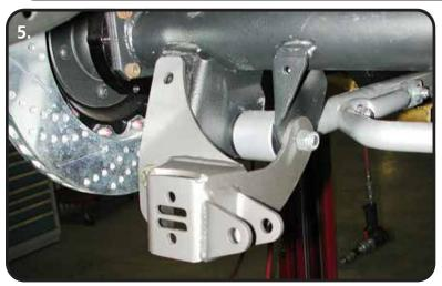
**5.** Remove the lower trailing arm mounting bolt. (Do one side at a time to keep the axle from rotating). Install the longer ½" x 3 ¾" bolt through the lower trailing arm from the outside in. Install the lower bracket over the bolt and secure with a ½" Nylok nut and flat washer. Snug the Hardware, but do NOT fully tighten at this time.
