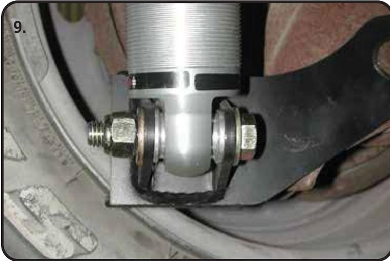
**9.** Fasten the CoilOver to the lower bracket using a 1/2" x 2 1/2" bolt, 1/2" flat washer, and Nylok nut. 1/2" I.D. aluminum spacers must be installed on each side of the bearing. Torque to 75 ftlbs.
