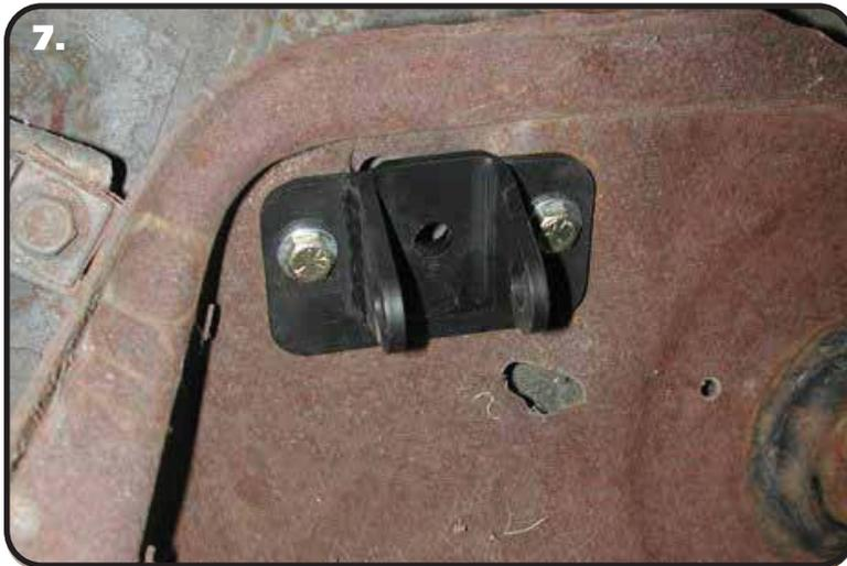
7. Fasten the new upper shock bracket into the factory shock location using the  $\frac{5}{16}$ " x  $1\frac{1}{4}$ " bolts, flat washers and Nylok nuts supplied. Torque to 17 ftlbs.
