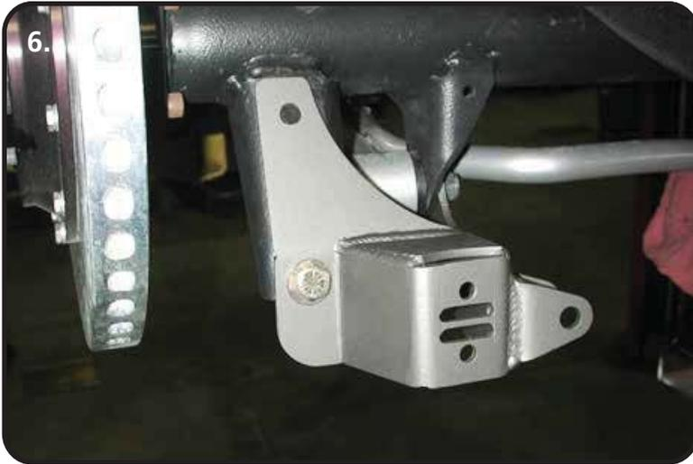
6. The lower bolt hole in the back of the bracket will align with the factory shock stud hole. Use a  $\frac{1}{2}$ " x  $1\frac{1}{2}$ " bolt, Nylok nut and flat washers. The upper hole must be drilled with a  $\frac{1}{2}$ " bit. The edge of the bracket should be parallel to the axle bracket. Use an centering punch and  $\frac{1}{8}$ " bit to drill a pilot hole. A  $\frac{1}{2}$ " x  $1\frac{1}{2}$ " bolt, Nylok nut and flat washers will be used here as well. Torque all hardware to 75 ftlbs.
