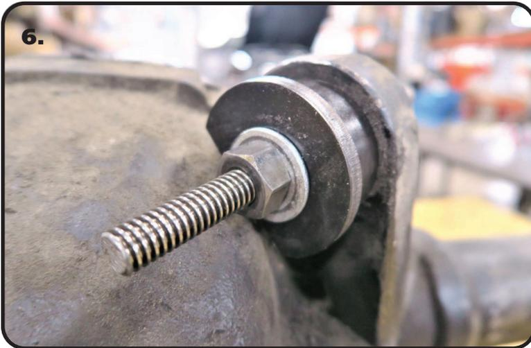
**6. 12 BOLT ONLY** The 2 5/8" Flat Sided Washer is made with a FLAT in it to clear the axle housing while installing the r-joint housing. You will need to position the Flat Sided Washer so it isn't hitting against the axle housing.
