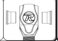
New R-Joints will be quite stiff (75-90 in/lbs breakaway torque) until they "break in" after a few miles of use. After the break in period they will move much more freely. Because the composite bearing race contains self lubricating ingredients, no additional lubrication is needed or desired. Any additional lubrication will only serve to attract more dirt and debris to the R-Joint and actually shorten its life.
