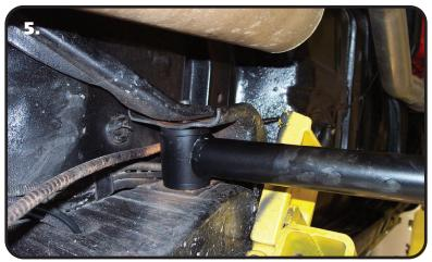
**5.** Attach to front on the lower StrongArm to the frame using the  $\frac{1}{2}$ " x 3  $\frac{1}{2}$ " bolts, flat washers and nylok nuts supplied.
