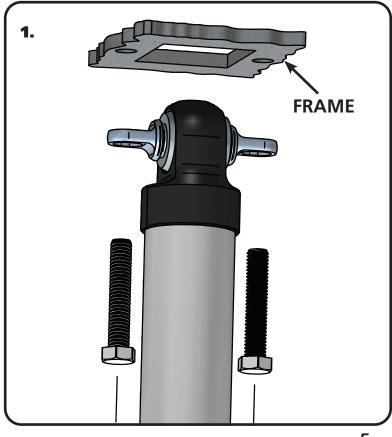
**1.** With the OEM Shock removed, install the Ridetech shock. Attach the Top of the Shock in the OEM Location using the OEM Hardware. It may be necessary to rotate the Trunnion to get it in the correct position. This can be done by sticking a screwdriver in one of the slots and spinning the trunnion in the shock bushing.
