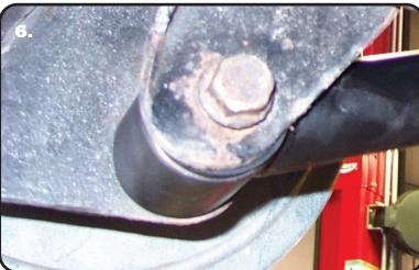
**3.** Attach to rear of the lower StrongArm to the frame using the  $\frac{1}{2}$ " x 3  $\frac{1}{2}$ " bolts, flat washers and nylok nuts supplied.
