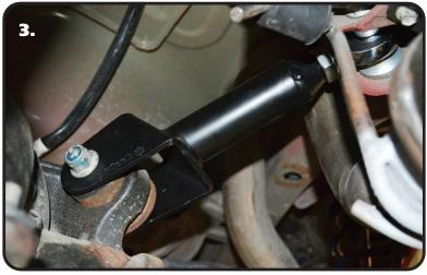
**3.** Install the R-Joint Spacers into the R-Joint End. Remove the OEM Upper Control Arms and replace them with the StrongArms.
