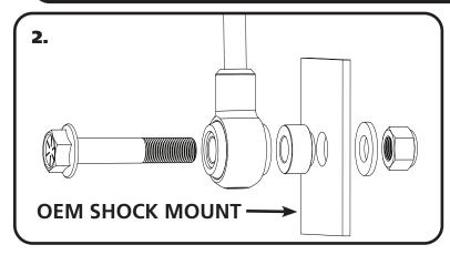
**2.** The Lower Shock is Bolted to the Lower OEM Mount using the supplied Cantilever Bolt Kit. Insert the Cantilever Bolt into the Shock Bushing. Next, Slide the Aluminum Spacer onto the Threads of the Cantilever Bolt. With the CoilSprings in place, Jack the Rear Differential up until the Shocks can be Bolted in place. Insert the Assembly into the OEM Shock Hole. Install the supplied Flat Washer and Nylok Nut onto the Threads and tighten.
