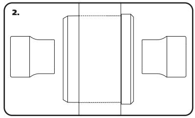
**2.** Install the Spacers by inserting the SMALL side of the SPACER into the Center Pivot Ball. Push them in until they bottom out and stop.
