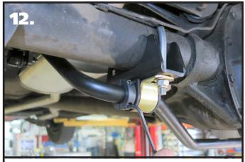
**12.** Install the locking rings on the outside of each bushing assembly. Use a hex key to take the locking ring apart. Reassemble it on the bar positioned next to the outside of the bushing assembly. Push the locking ring up against the bushing assembly and tighten.
