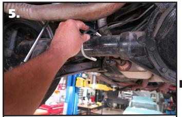
**5.** Install the u-bolts onto the axle tube with the threads pointing down. You may need to raise the brake lines in the area of the u-bolts. The u-bolts will be approximately 23 1/2" apart and equal distance on each side from the brake backing plates.
