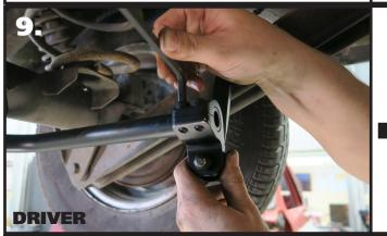
**9.** Apply Antisieze to (4) 3/8"-16 x 7/8" socket head cap screws and thread them into the clamp-on ends. Install a clamp-on end on each end of the bar. The end link mounting hole should be mounted to the outside of the bar and pointing down. Start with the mount flush with the end of the bar.
