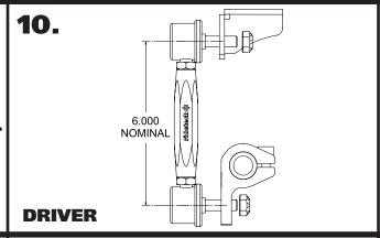
**10.** Assemble the end links. Set the linkage to 6" center to center with the threaded studs pointed opposite directions. Snug the jam nuts against the center adapter. Attach the sway bar linkage to the clamp-on mount using the hardware on the linkage. Attach the correct tab to the top of the linkage with the gusset to the front. Use **Diagram 10** as a reference. Attach the linkages and tab to both sides.
