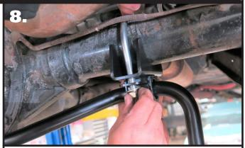
**8.** Hold the sway bar in position on the car with the center bend toward the ground. Install a 7/16" flat washer & 7/16"-20 nylok nut on the threads of the u-bolts. Snug the hardware down and verify that it is centered and the axle mounts are level. Torque the u-bolt hardware.
