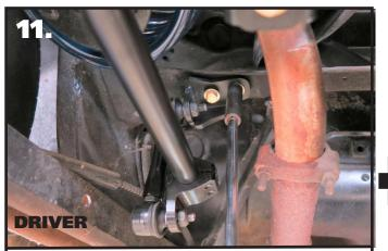
**11.** Swing the tab up to the frame, keeping the linkage straight from side to side. Use the tab to mark the location of the holes that will need to be drilled. Drill the holes with a 3/8" drill bit. Install a 3/8" flat washer on each of (2)  $3/8"-16 \times 1 \ 1/4"$  hex bolts and install them through the bracket and drilled holes. Install a 3/8" flat washer & 3/8"-16 nylok nut on each bolts sticking through the frame. Torque the hardware and repeat on the other side.
