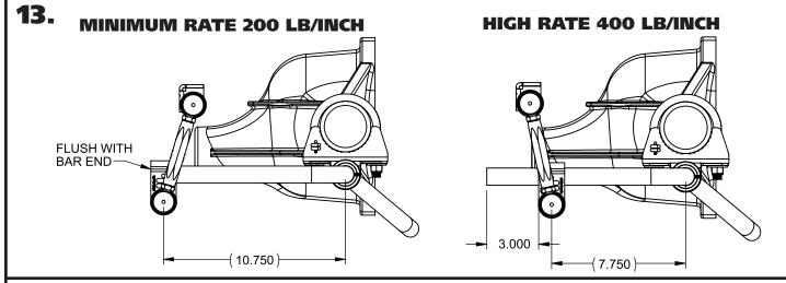
**13.** We recommend getting the swaybar as level as possible at ride height and with no preload. Both of these steps are done by adjusting the end links. These end links can be adjusted from 6" to 6 3/4". Disconnect the end links from the swaybar and adjust one side to get the swaybar level. Reattach the end link to the swaybar and adjust the 2nd end link so that it goes in and out of the clamp-on mount with ease. This will be zero preload.
