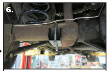
**6.** Install an axle bracket onto each u-bolt with the flat side to toward the ground. The "teeth" of the mount should touch the axle tube.
