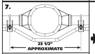
**7. Diagram 7** illustrates the correct installation of the sway bar. Again, the axle brackets will be approximately 23 1/2" from center to center. The mounts should be spaced equal amounts from the brake backing plates, centering the sway bar on the axle.
