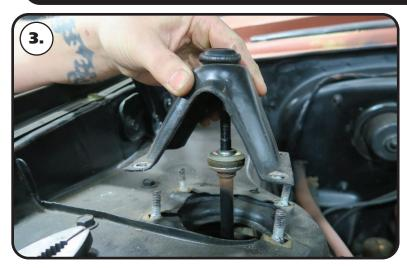
**3.** The OEM upper shock mount will need to be removed from the car. Remove the upper shock nut and unbolt the mount.
