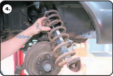
**4.** If you haven't done so already, remove the shock spring assembly out of the car.
