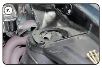
7. The kit includes an upper spacer due to different metal thicknesses at the upper shock mounting area. Place the upper spacer on top of the shock tower with the opening to the FRONT of the car and the curves side toward the engine. The mounting holes will align with the outer slots of the upper shock mount.
