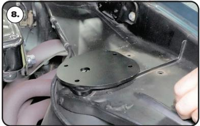
**8.** The upper mounting plate sits on top of the spacer. The mounting holes will align with the holes in the spacer plate.
