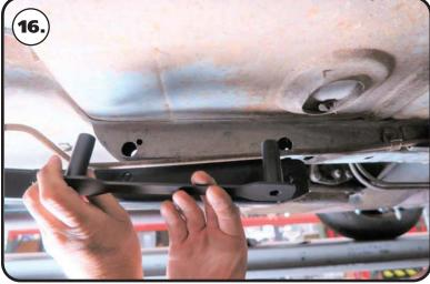
**16.** The kit includes clamp spacer plates to help sandwich the frame rail without crushing it. The bungs of the clamp spacer will need to be inserted into the 3/4" holes.
