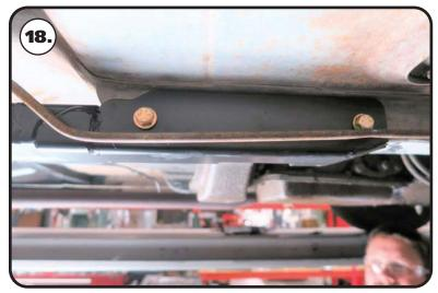
**18.** Slip the front of the connector up over the frame rail and clamp plate. Install a 7/16" flat washer on each of (2) 7/16"-14 x 4" hex bolts. Insert the bolts into the 2 mounting holes.
