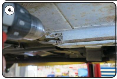
**4 & 5.** Any fuel line or brake line clamps that are on the frame rail in the area of the transmission crossmember, will need to be removed from the frame rail. Some will need to be removed by drilling the center.
