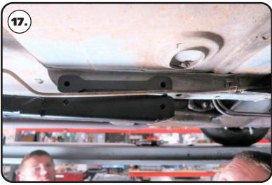
**17.** Push the clamp spacer tight against the frame.
