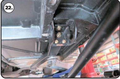
**22.** Install a 3/8" flat washer on each of (2) 3/8"-16 x 1 1/4" hex bolts. Insert the bolt/ washer through the (2) lower mounting holes of the subframe connector and into the leaf spring mount.
