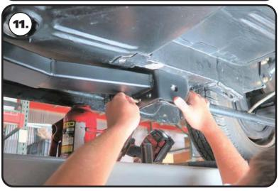
11. Install a 3/8" flat washer on a (1) 3/8"-16 x 1 1/4" hex bolt. Insert the bolt/washer through one of the rear mounting holes of the subframe connector and into the leaf spring mount. Install a 3/8" flat washer and 3/8"-16 nylok nut on the bolt. Leave the hardware loose for the time being.
