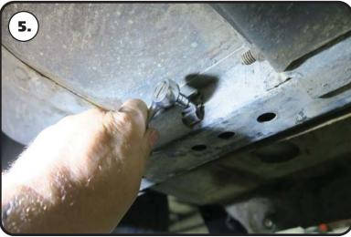
**5.** Some clamps may be screwed to the frame. Remove the center screw to remove the clamp.
