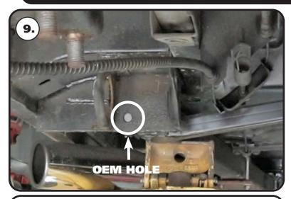
**9.** The subframe connector uses an OEM hole in the OEM leaf spring mount. The other 2 holes will need to be drilled. The subframe connector can be used to mark the 2nd bottom hole. A template is provided on **Page 10** for drilling the top hole.
