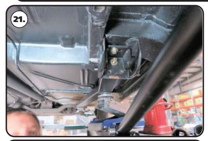
**21.** Install a 3/8" split lock washer & 3/8" SAE flat washer on (1) 3/8"-16 x 1 1/4" hex bolt. Insert the bolt/washers in the top hole, threading it into the rear of the subframe connector. Do not tighten until all of the hardware is installed.
