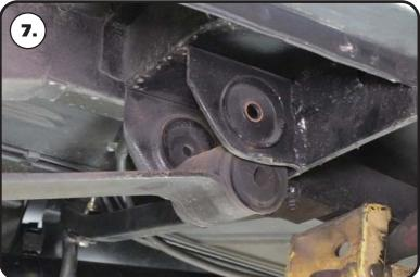
**7.** Drop the front of the leaf spring down to give access to the front of the leaf spring mount.
