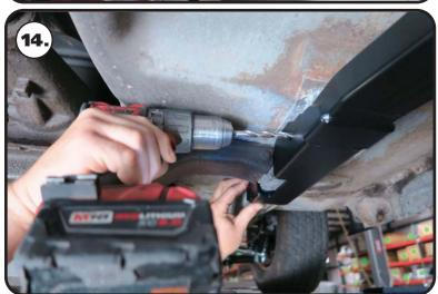
**14.** MAKE SURE THE SUBFRAME CONNECTOR IS PUSHED UP TIGHT AGAINST THE FRAME. Use the subframe connector as a template to drill the inner and outer holes to 7/16"
