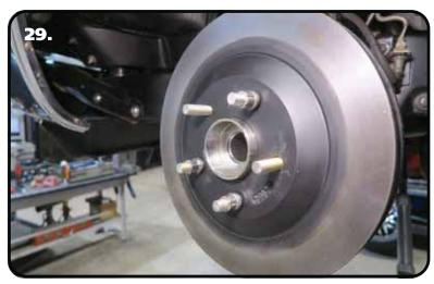
**29.** Install the rotor on the hub. Thread some lug nuts on the threads of the hub to hold the rotor tight on the hub.
