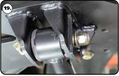
**19.** Install another eccentric eliminator on the threads of the bolt. Make sure the plate is orientated the same as the other plate. Install a 1/2" flat washer and 1/2"-20 nylok nut on the bolt. Repeat for the 2nd bushing. Torque the hardware to 120 ft-lbs.
