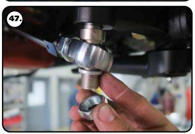
**47.** Install the 5/8" ID x .125" spacer on the stud followed by a 5/8"-18 mechanical locking nut. Torque to 45 ft-lbs.
