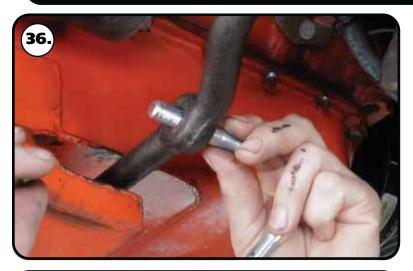
**36.** The SMALL tapered studs will get installed into the factory centerlink with the taper going into the centerlink, a 7/16" castle nut is used to attach it to the centerlink. The straight shank will point to the front of the car.
