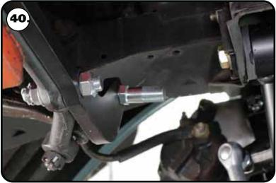
**40.** The studs with the short hex get installed into the centerlink adapter. The short side goes into the adapter attached with the 5/8"-18 thin top lock nut, with the long side of the stud pointing forward.
