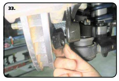
**33.** Insert the steering arm inserts into the spindle using the correct orientation from the details above.
