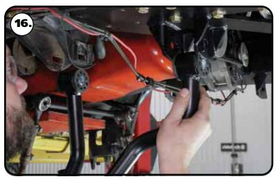
**16.** Insert the lower control arm into the mounts. The rear bushing goes into the OEM mount. The front busing gets installed into the mount on the new lower control arm plate. Align the through hole of the bushing with the slots in the mounts.
