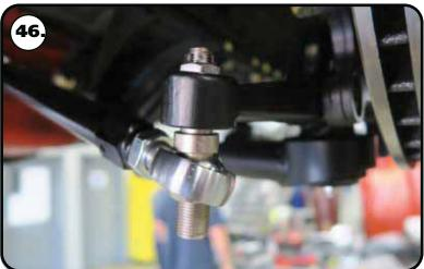
**46.** Install a 5/8" ID x 3/8" spacer on the steering arm stud, followed by the outer end of the tie rod.
