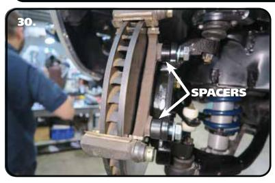
**30.** The kit includes spacers that will be installed between the caliper bracket and caliper mount. Install a M14 flat washer on each of (2) M14-2.0 x 45mm hex bolts. Insert the bolts through the caliper bracket, installing a spacer on each bolt. Line the caliper mount up with the hardware and thread in the bolts.
