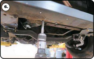
**6.** The remainder of the rivets will need to be removed from the frame of the car.
