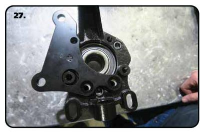
**27.** The caliper brackets are side specific. They have a D & P stamped in them. Lay the correct side caliper bracket on top of the shims, aligning the mounting holes with the mounting holes of the bracket. The counter sunk holes should facing up.
