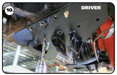
**10.** Use a 7/16" drill bit to drill the (4) holes in the frame rail that don't exist.
