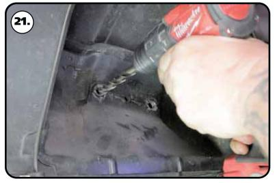
**21.** The OEM upper control arm holes need to be drilled out using a 1/2" drill bit.
