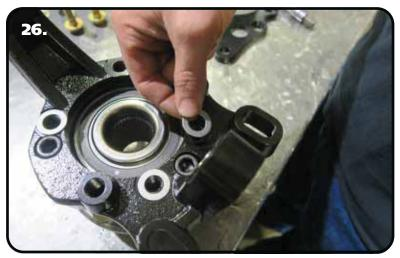
**26.** Lay a .062" thick, 1/2" ID shim on each of the caliper brackets (3) mounting holes.
