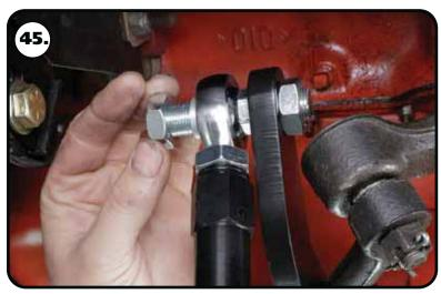
**45.** Install the 5/8" ID x .125" spacer on the stud followed by a 5/8"-18 mechanical locking nut. Torque to 45 ft-lbs.
