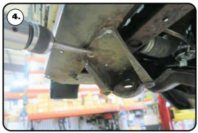
**4.** With the "+" cut in the head of the rivet, chisel the head of the rivet off. The head of the rivet should come off in 4 pieces.
