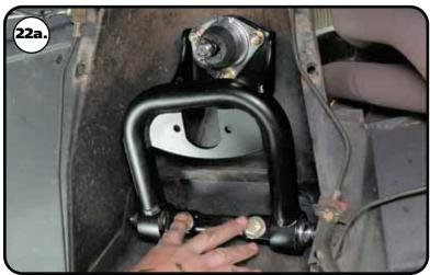
**22a. Steps 22a & 22b** illustrate mounting the upper control arm. The upper StrongArm gets bolted to the body using ½"-20 x 2 ½" bolts & flat washers. **The ARROW points to the front of the vehicle.**
