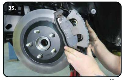
**35.** Install the brake pads and caliper.
