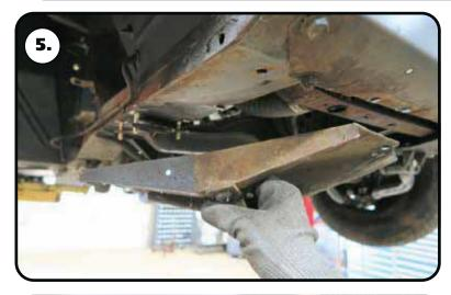
**5.** With the rivet heads removed, the strut rod mount can be removed from the car.
