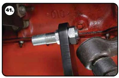
**41.** Install the 5/8"-18 **THIN** mechanical locking nut on the threads of the stud sticking through the centerlink adapter and torque to 45 ft-lbs.
