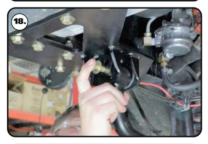
**18.** Install a 1/2" flat washer on each of (4) 1/2"-20 x 4" hex bolt. Insert the bolt in the eccentric eliminator plate. Install the assembly in the lower control arm mount. Repeat for the 2nd bushing.
