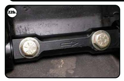
**22b.** Hold the arm in place and install the bolt/ washers. Install a 1/2" split lock washer and 1/2"-20 nut on the threads of the bolts that are sticking through the shock tower. Torque the hardware to 110 ft-lbs.
