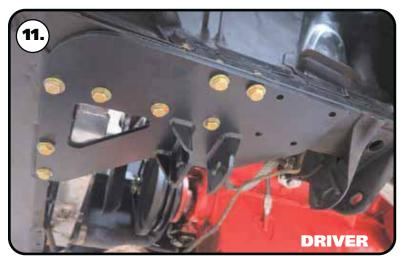
**11.** Install a 7/16" flat washer on each of (4) 7/16"-14 x 1 1/4" bolts. Insert the bolts/ washers in the holes that align with the holes that were just drilled. The threads of the bolts need to be pointing up. Install a 7/16" flat washer and 7/16"-14 nylok nut on each of the bolts. Torque the bolts to 80 ft-lbs. Repeat Step 8-12 on the other side.
