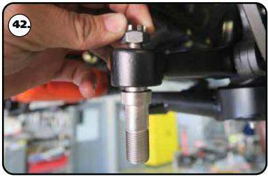
**42.** Install the stud with the round flange into the steering arm with the taper going into the steering arm. Torque the nuts to 35 ft-lbs and tighten as needed to align cotter pin hole and install cotter pin.
