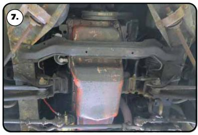
**7.** The crossmember will need to be removed from the car. **The crossmember will be reinstalled later.**
