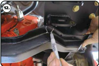
**13.** The crossmember will need to be notched to clear the lower control arm mount. Hold the crossmember up in position to see where you will need to notch it.
