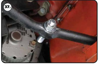
**37.** Torque the nuts to 35 ft-lbs and tighten as needed to align cotter pin. Install cotter pin and bend the ends.
