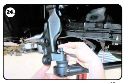
24. The spindles included in this kit are identical for each side. They are not side specific until the steering arm is attached. Install the spindle on the lower ball joint pin. Torque the ball joint castle nut to 65 ft-lbs and tighten to align the cotter pin holes. Install the cotter pin in the ball joint pin hole and bend the ends of the cotter pin to hold it in place. Install the grease zerk supplied with the ball joint.
