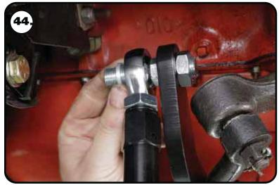
**44.** Install one end of the tie rod onto the stud of the centerlink adapter.
