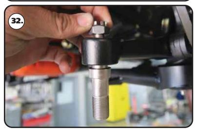
**32.** Install the stud with the round flange into the steering arm with the taper going into the steering arm. Torque the nuts to 35 ft-lbs and tighten as needed to align cotter pin hole and install cotter pin.
