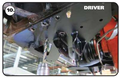
Use **Images 8 - 12** as a guide to install the lower control arm mounts.
