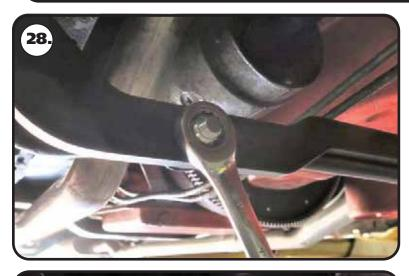
**28.** Install the draglink adapter on the studs sticking out of the OEM draglink. Install a 1/2"-20 mechanical locking nut on the threads of each stud sticking through the draglink adapter. Torque the nuts to 50 ft-lbs.
