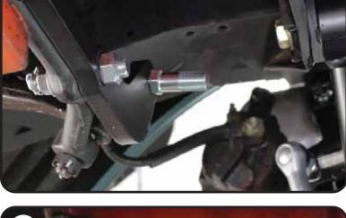
**30.** Install the 5/8"-18 **THIN** mechanical locking nut on the threads of the stud sticking through the centerlink adapter and torque to 45 ft-lbs.
