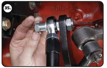
**35.** Install the 5/8" ID x .125" spacer on the stud followed by a 5/8"-18 mechanical locking nut. Torque to 45 ft-lbs.
