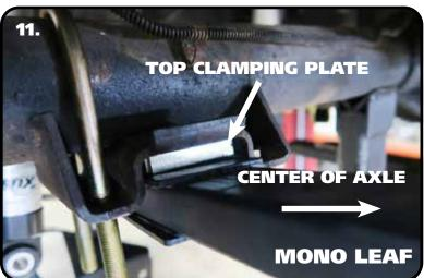
**11.** Remove the OEM Hardware from the OEM leaf spring mount, it will be replaced with hardware supplied in the kit. The new Hardware includes (1) 7/16 U Bolt, (2) 7/16"-20 x 2 1/4" Hex Bolts, (4) Flat Washers, & (4) 7/16-20 Nylok Nuts per side. The U Bolt will replace the outer OEM hardware, the 7/16" x 2 1/4" bolts replace the inner OEM hardware. Install the U Bolt and Hex Bolts.
