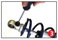
Before the upper spring mount can be installed screw the adjuster knob on the upper eye mount to the firmest setting (clockwise) as seen in figure 3. Then remove the Knob by holding it while removing the center screw.
