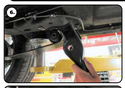
**6.** Remove the OEM leaf spring mount from the front of the leaf spring. Retain the leaf spring hardware for reassembly. Replace the OEM U-nuts in the floor pan and frame rail with the new ones supplied in the hardware kit.
