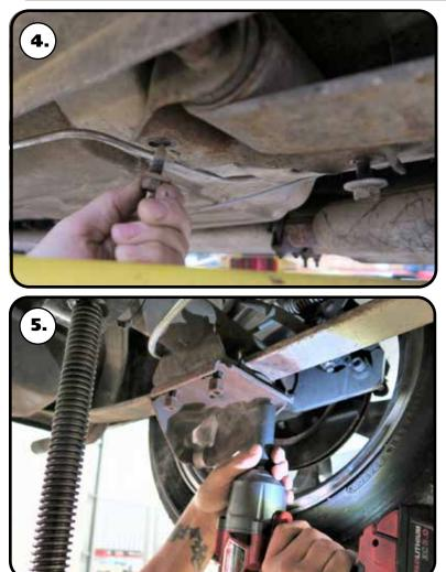
**4.** Support the center of the differential with a jack. Remove the 3 bolts from the OEM leaf spring mounts. Do this for both sides.
