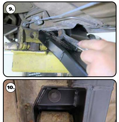
**9.** Attach the rear of the subframe connector to the front of the leaf spring. Install the leaf spring bolt from the inside of the car with the nut to the outside. The leaf spring bolt will need to be tightened before the subframe connector is installed.
