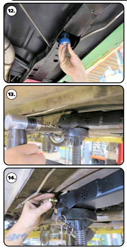
**12.** Push the front subframe connectors up against the OEM subframe. Reinstall the OEM body bushing/bolt.
