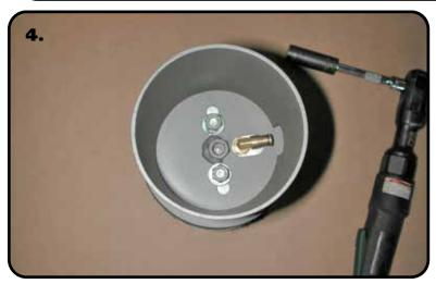
**4.** Apply thread sealant to the air fitting and screw it into the air spring. Assemble the upper cup bracket to the air spring, using 3/8"-16 Nylok nuts and 3/8" flat washers. Torque the 3/8" nuts 15-20 ftlbs.
