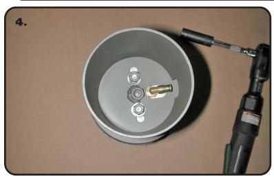
**4.** Apply thread sealant to the air fitting and screw it into the air spring. Assemble the upper cup bracket to the air spring, using 3/8"-16 Nylok nuts and 3/8" flat washers. Torque the 3/8" nuts 15-20 ftlbs.
