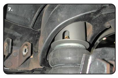
7. Place the air spring assembly into the coil spring pocket with the tab on the side of the cup aligning with the factory bump stop mount. The stud should poke through the hole in the upper coil spring pocket. Some cars may not have this hole and it must be drilled with a 7/16" drill bit. Fasten with a 7/16" Nylok nut and flat washer. Torque 25-35 ft-lbs.
