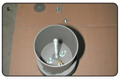
**5.** Thread the 6" stud into the nut in the bottom of the cup.
