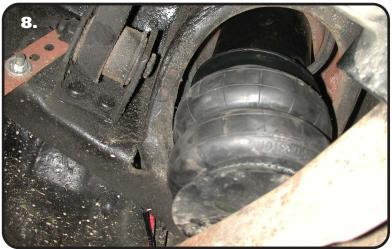
**8.** Slide the lower plate between the air spring and the lower arm. It is held tight with a 3/8" x 3/4" bolt with flat washer and lock washer. Torque the 3/8" bolt to 15-20 ftlbs.
