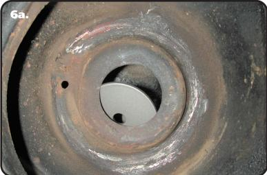
**6a & 6b** The large washer needs to be installed on the TOP side of the frame at the coil spring pocket.
