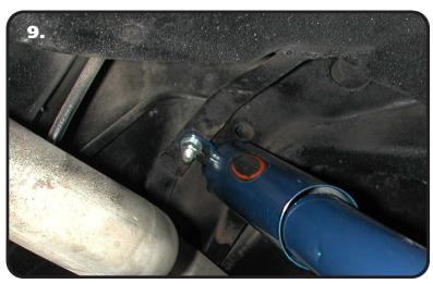
**9.** Attach shock T-Bar to frame using 5/16" x 1" bolts, Nylok nuts and flat washers. Torque to 17 ft-lbs.
