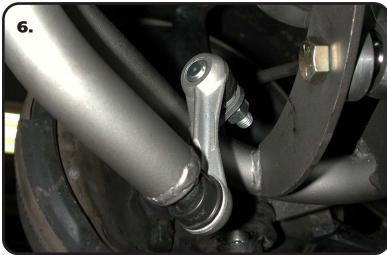
**6.** The other end of the PosiLink will attach to the tab on the StrongArm using a flat washer on each side of the tab and M12-1.75 nylok nut.
