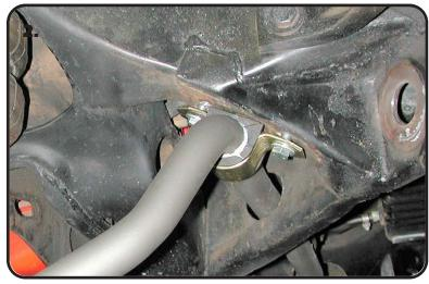
**2.** Lubricate the sway bar busing with the lithium grease supplied. Install the new polyurethane bushing and strap over the sway bar.
