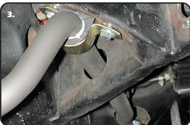
**3.** Clamp the sway bar up to the frame using a couple "C" clamps. The sway bar should be centered in the hole through the frame.
