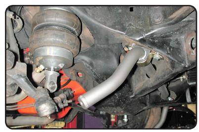
**1.** Slide the sway bar though the same holes in the frame that the factory bar went through. The sway bar needs installed with the center dropping down toward the ground to clear the engine.
