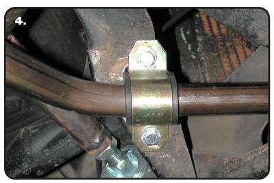
**4.** The factory bolt holes may not line up with the new strap. If not, two new holes must be drilled with a 3/8" bit. Secure the assembly with two 3/8" x 1 1/4" bolts, flat washers and Nylok nuts.
