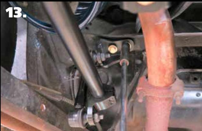
**13.** Swing the tab up to the frame, keeping the linkage straight from side to side. Use the tab to mark the location of the holes that will need to be drilled. Drill the holes with a 3/8" drill bit. Install a 3/8" flat washer on each of (2) 3/8"-16 x 1 1/4" hex bolts and install them through the bracket and drilled holes. Install a 3/8" flat washer & 3/8"-16 nylok nut on each bolts sticking through the frame. Torque the hardware and repeat on the other side.
