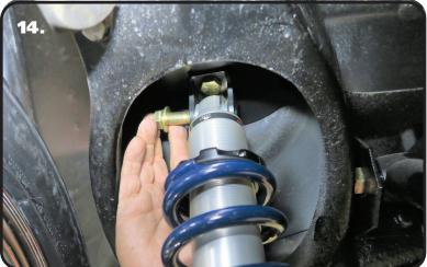
**14.** Insert the shock into the upper mount, lining up the holes of the mount and shock bearing/spacers. Install a 1/2" flat washer on a  $1/2"-13 \times 2 1/2"$  bolt. Insert the bolt/ washer into the upper mount/shock. Install a 1/2" flat washer and 1/2"-13 nylok nut and Torque to 50 ftlbs.
