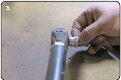
**3.** Install the <sup>3</sup>⁄<sub>4</sub>" jam nut onto the end of the R-Joint end, then screw R-Joint end into the end of the panhard bar. Set the Panhard Bar to 35.750". You may need to readjust it after getting the car set at ride height, but this is a good starting point. Press the SMALL diameter of the 9/16"I.D. R-Joint spacers into each side of the center ball of the remaining R-Joint. Push the spacers in until they bottom out in the center ball.
