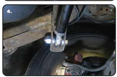
**4.** Insert the R-Joint Housing end of the panhard bar into the OEM frame mount. Align the align hole in the R-Joint end with the holes in the OEM mount. Install a 9/16" flat washer on a 9/16"-18 x 3" hex bolt and insert in into the aligned holes. Install a 2nd 9/16" washer followed by a 9/16"-18 nylok nut on the threads of the bolt sticking through the frame. Torque to 95 ftlbs.
