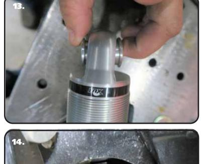
**14.** Insert the shock into the upper mount, lining up the holes of the mount and shock bearing/spacers. Install a 1/2" flat washer on a  $1/2"-13 \times 2 1/2"$  bolt. Insert the bolt/ washer into the upper mount/shock. Install a 1/2" flat washer and 1/2"-13 nylok nut and Torque to 50 ftlbs.
