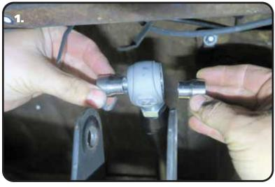
**1.** Insert the small diameter of the R-Joint Spacers into the center ball of the R-Joint. Insert the R-Joint/Spacers into the OEM mount of the differential.
