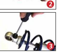
Before the upper spring mount can be installed screw the adjuster knob on the upper eye mount to the firmest setting (clockwise) as seen in figure 3. Then remove the Knob by holding it while removing the center screw.
