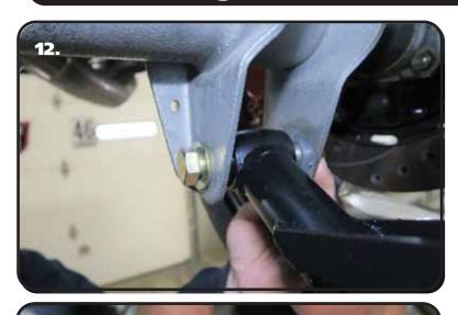
**12.** Install a 5/8" flat washer on a 5/8"-18 x 4" bolt. Insert the bolt/washer through the mounting hole. Install a 5/8" flat washer and 5/8"-15 nylok nut on the threads of the bolt sticking through the axle mount. Tighten the hardware to eliminate any gaps
