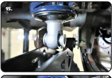
**15.** Insert the LONG shock bearing t-bushings into the bearing of the shock eyelet. The SMALL diameter of the t-bushings will insert into the shock bearing.
