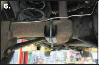
**6.** Install an Axle bracket onto each u-bolt with the flat side to toward the ground.
