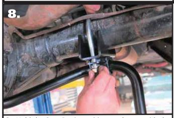
**8.** Hold the SwayBar in position on the car with the center bend toward the ground. Install a 7/16" Flat Washer & 7/16"-20 Nylok Nut on the threads of the u-bolts. Snug the hardware down and verify the swaybar is centered and the axle mounts are level. Torque the u-bolt hardware.
