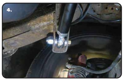
**5.** Check the side to side dimension between the tire and quarter panel with the car at ride height. You may need to adjust the panhard bar to center the axle at ride height.
