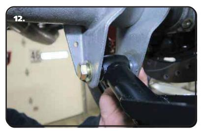
**12.** Install a 5/8" flat washer on a 5/8"-18 x 4" bolt. Insert the bolt/washer through the mounting hole. Install a 5/8" flat washer and 5/8"-15 nylok nut on the threads of the bolt sticking through the axle mount. Tighten the hardware to eliminate any gaps
