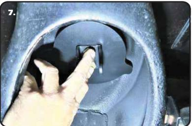
7. Position the Shock Mount/Plate up into the frame, holding the shock mount and hardware in place. Positon the mount with the tabs to the front of the car and Ridetech Icon toward the wheel. You will need to align the upper clamp plate with the bolts that are sticking up through the frame.
