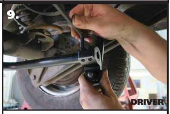
**9.** Apply Antisieze to (4) 3/8"-16 x 7/8" Socket Head Cap Screws and thread them into the Clamp-On Ends. Install a clamp-on end on each end of the bar. The End Link mounting hole should be mounted to the outside of the bar and pointing down. Start with the mount flush with the end of the bar.
