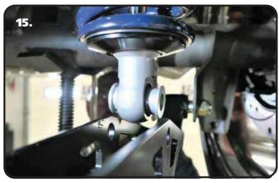
**15.** Insert the LONG shock bearing t-bushings into the bearing of the shock eyelet. The SMALL diameter of the t-bushings will insert into the shock bearing.
