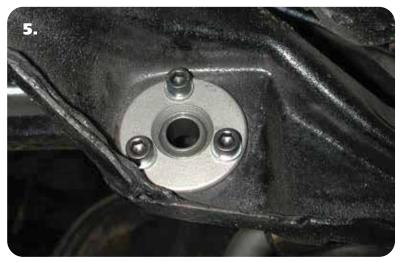
**5.** Using the bearing retainer as a template; drill three 3/8" holes in the frame to secure the assembly. Use three 3/8" x 1 ¼" SHCS and lock washers to secure the assembly. Torque to 30 ft-lbs.
