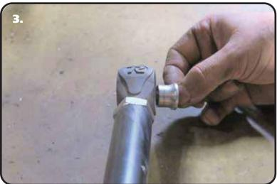
**3.** Install the ¾" jam nut onto the end of the R-Joint end, then screw R-Joint end into the end of the panhard bar. Set the Panhard Bar to 35.750". You may need to readjust it after getting the car set at ride height, but this is a good starting point. Press the SMALL diameter of the 9/16"I.D. R-Joint spacers into each side of the center ball of the remianing R-Joint. Push the spacers in until they bottom out in the center ball.
