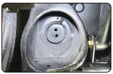
**5. Image 5** shows the Upper Clamp Plate in poistion as looking at it from the bottom side of the frame. Don't worry about the orientation of the bolt holes. You will position it correctly during the intallation of the Upper Shock Mount.
