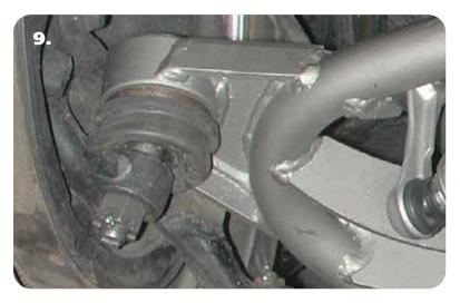
**9.** Attach the spindle to the control arms.
