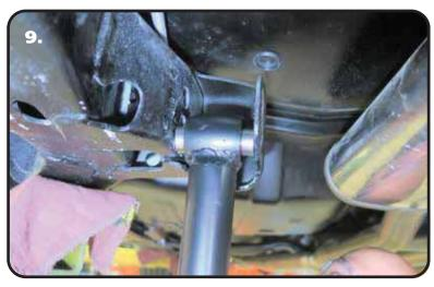
**9.** The Lower Control Arm has the bottom CoilOver mount built in. It will need to be installed with the CoilOver mount up and to the rear of the car. Install a 5/8" ID R-joint Spacer into the front R-joint. The Small Diameter goes into the R-joint. Slide the R-joint into the OEM lower control arm mount. Align the holes in the frame with the thru-hole of the R-Joint.
