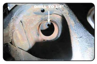
**1.** Drill the OEM shock hole out to 3/4". This can be done with a Unibit.
