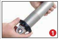
First, using the supplied lower adjuster nut (803-00-199) thread the nut onto the shock from the bottom side as seen in figure 1. Remove the plastic pellet that is in the split of the adjuster nut.
