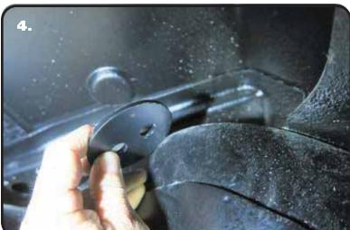
**4.** The The Upper Clamp Plate needs to be placed on the top side of the OEM coilspring pockect. It will fit down in the recessed area of the coilspring pocket. Use **Images 4 & 5** as a reference to install the upper clamp plate.
