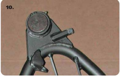
**10.** Thread the 3/8"-16 nut onto the 3/8"-16 x 1 ¼" bolt. Thread it into the front hole of the ball joint plate. You will need to adjust the steering stop to suite your needs. This setting will vary depending on wheel and tire size and other suspension components. Torque to 16 ft-lbs.
