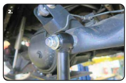
**2.** Install a Narrow 5/8" ID R-joint Spacers into each side of the R-joint of either end of the Panhard Bar. The Small Diameter goes into the R-joint. Slide the R-joint onto the stud and fasten in place with a 5/8" flat washer and 5/8"-18 thin jam nylok nut. Torque to 95 ftlbs.
