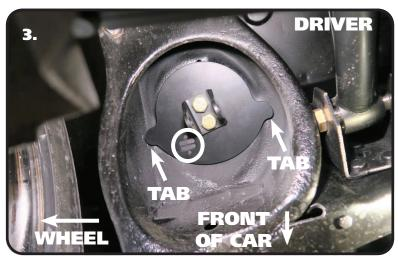
**3.** This kit contains a Upper Shock Mount setup that is designed to be mounted in a specific orientation. **Image 3** illustrates the proper orientation of the upper mount, we will cover the installation in the next steps. The upper mount is installed in the OEM coilspring pocket with the TABS of the upper plate to the front of the car. The Ridetech Icon(CIRCLED) needs to be toward the wheel. See **Image 3**.
