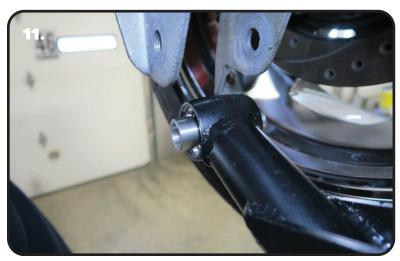
**11.** Install the R-joint spacers into the rear R-Joints. Slide the rear of the lower control arm into the axle mount. Line up the mounting holes in the axle mount with the thru-hole of the R-joint.
