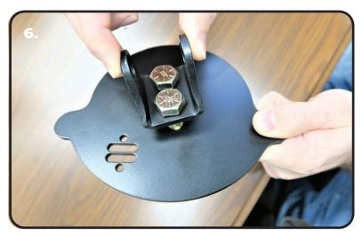
**6.** The Upper Mount Assembly is attached to the frame using (2) 1/2"-13 x 1 1/2" Bolts. Insert the bolts through the shock mount and through the upper plate.
