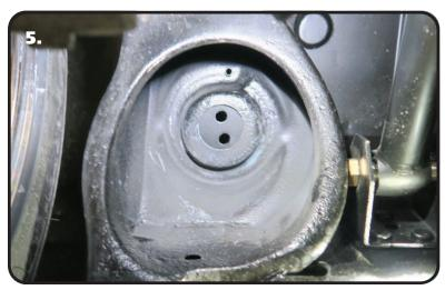
**5. Image 5** shows the Upper Clamp Plate in position as looking at it from the bottom side of the frame. Don't worry about the orientation of the bolt holes. You will position it correctly during the installation of the Upper Shock Mount.
