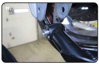
**11.** Install the R-joint spacers into the rear R-Joints. Slide the rear of the lower control arm into the axle mount. Line up the mounting holes in the axle mount with the thru-hole of the R-joint.
