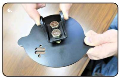
**6.** The Upper Mount Assembly is attached to the frame using (2) 1/2"-13 x 1 1/2" Bolts. Insert the bolts through the shock mount and through the upper plate.
