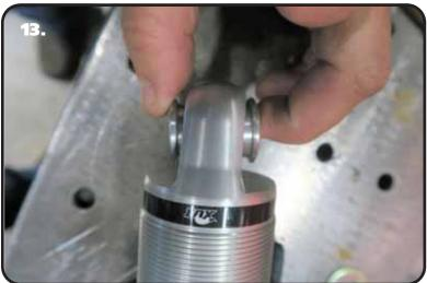
13. Refer to the CoilOver instructions that are included with the CoilOvers for proper CoilOver assembly. Insert the SHORT shock bearing t-bushings into the bearing of the **shock body**. The SMALL diameter of the t-bushings will insert into the shock bearing.
