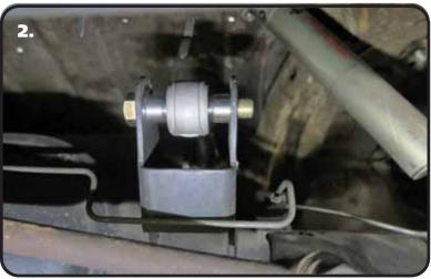
2. Install a 5/8" flat washer on a 5/8"-18 x 4" hex bolt through the mount and control arm R-Joint. Install a 5/8" flat washer, followed by a 5/8"-18 nylok jam nut onto the threads of the bolt. Tighten the hardware enough to eliminate any gaps.
