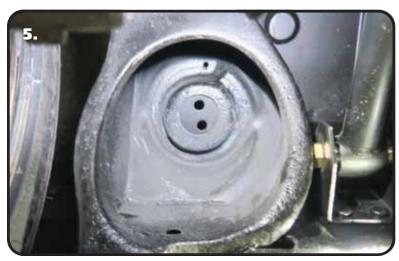
**5. Image 5** shows the Upper Clamp Plate in position as looking at it from the bottom side of the frame. Don't worry about the orientation of the bolt holes. You will position it correctly during the installation of the Upper Shock Mount.
