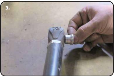
**3.** Install the ¾" jam nut onto the end of the R-Joint end, then screw R-Joint end into the end of the panhard bar. Set the Panhard Bar to 35.750". You may need to readjust it after getting the car set at ride height, but this is a good starting point. Press the SMALL diameter of the 9/16"I.D. R-Joint spacers into each side of the center ball of the remaining R-Joint. Push the spacers in until they bottom out in the center ball.
