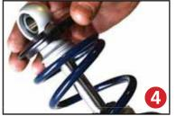
Once the knob is removed slide a Delrin washer over the eyelet. Next, slide the upper spring mount (803-00-199) over eyelet as seen in figure 4.
