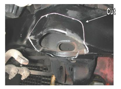
3. To allow clearance for the air spring a portion of the frame to the outside of the coil spring pocket must be removed. This can be accomplished using a plasma cutter or die grinder with a cut off wheel. Grind all edges smooth after finished.
