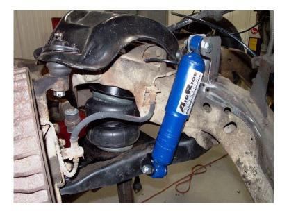
1. The upper shock mount must be welded to the frame. It may need to be cut down to match the stroke of the air spring and suspension. Make sure that when the suspension is fully compressed that the shock is about 1/4" from being fully compressed.
