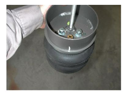
5. Place the upper cup bracket on top of the air spring and fasten with two 3/8" nylok nuts and flat washers. Thread the 7/16 stud into the nut in the bottom of the cup.
