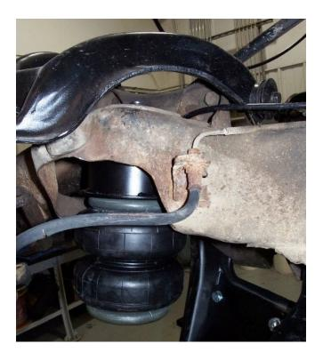
7. Place the air spring assembly into the coil spring pocket with the stud sticking through the factory shock hole in the frame.
