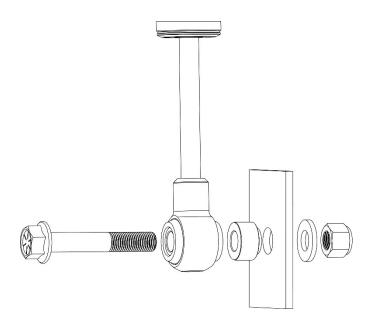
1. Attach the upper T-bar to the frame in the oem location using the supplied 5/16 x 1" USS bolts, washers and Nylok nuts.
