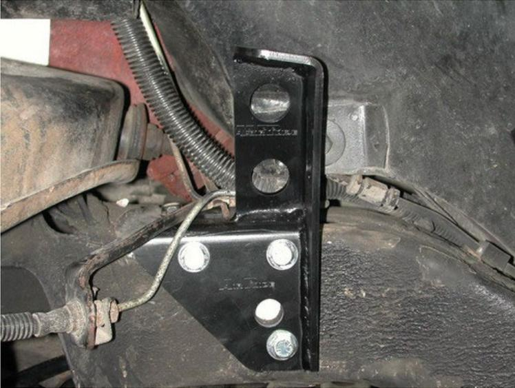
1. The shock bracket must be mounted first. It bolts right behind the upper arm and locates off the large hole in the frame and in the bracket. The brake line bracket must be removed and then reinstalled over the top of the shock bracket. The shock bracket is secured with 1 ¼" x ¾" bolts with Nylok nuts and flat washers.
