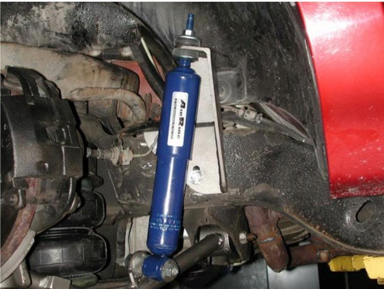
2a. **If using the factory lower arm;** a .625" hole must be drilled in rear leg of the lower arm for the cantilever pin. This hole should be approximately 9" from the ball joint.
