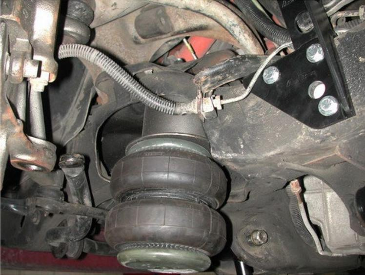
1. Some trimming around the outside of the coil spring pocket is required for air spring clearance. This arc should be approximately 2" tall by 5" long. This is best done with a cutoff, sawzall, or plasma cutter.
