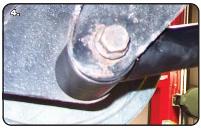
**4.** Attach to rear of the lower StrongArm to the frame using the  $\frac{1}{2}$ " x 3  $\frac{1}{2}$ " bolts and Nylok nuts supplied.
