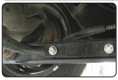
**2.** If your lower arm doesn't have any internal support at the mounting holes, insert the Supplied Spacer into the inside of the Control Arm at the Hole Locations. These Spacers will get Clamped in place by the Mounting Hardware after the SwayBar is installed. These can be welded in place if desired.
