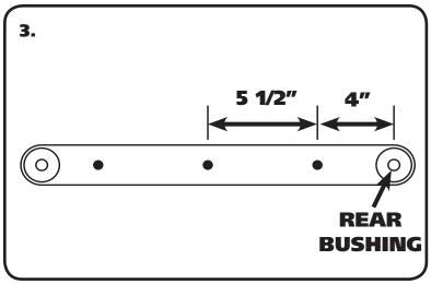
1. Every car we have worked with had the holes for a swaybar. They had 3 holes, but the front hole isn't used to mount the swaybar. If your Car has no holes, measure forward 4" from the center of the Rear Bushing and make a mark centered top to bottom. Next measure forward 5 1/2" from your first mark and mark the second hole centered top to bottom. Drill the locations with a 7/16" Drill Bit going through both sides of the Arm. Repeat for both Arms.
