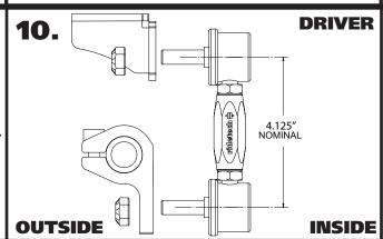
**10.** Assemble the end links. Set the Linkage to 4 1/8" center to center with the threaded studs pointed the same direction. Snug the jam nuts against the center adapter. Attach the SwayBar Linkage to the Clamp-On Mount using the hardware on the linkage. Attach the correct tab to the top of the linkage with the gusset to the front. Use **Diagram 10** as a reference. Attach the linkages and tab to both sides.
