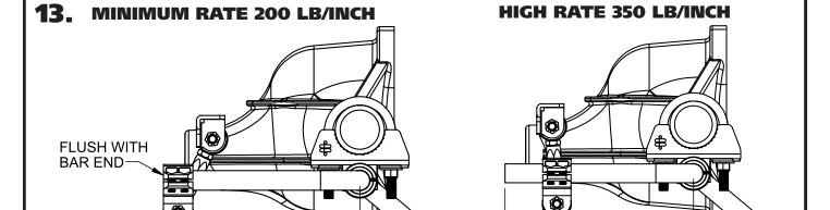
**13.** We recommend getting the swaybar as level as possible at ride height and with no preload. Both of these steps are done by adjusting the end links. These end links can be adjusted from 4 1/8" to 4 7/8". Disconnect the end links from the swaybar and adjust one side to get the swaybar level. Reattach the end link to the swaybar and adjust the 2nd end link so that it goes in and out of the clamp-on mount with ease. This will be zero preload.
