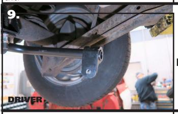
**9.** Thread (2) 3/8"-16 x 7/8" Socket Head Cap Screws into each of the Clamp-On Ends. Install a clamp-on end on each end of the bar. The End Link mounting hole should be mounted to the inside of the bar and pointing down. Start with the mount flush with the end of the bar.
