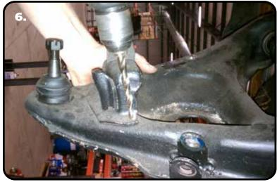
**6.** Use a drill to drill the spot welds out of the OEM bumpstop/steering stop. Just drill through the mount. Do NOT drill through the control arm. We recommend cleaning the area up after removing it and paint it to keep the area from rusting.
