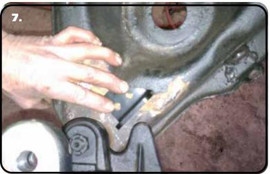
7. Use the Image as a reference for placing the steering stop. It should be parallel with the rear edge of the control arm. You want the steering stop of the spindle to hit the steering stop before the steering box hits the internal stop. Use the stop as a template to drill (2) 3/8" holes in the control arm. Attach the stop using (2) 3/8"-16 x 1" bolts, (4) 3/8" flat washers, & (2) 3/8"-16 nylok nuts. Torque to 30 ft-lbs.
