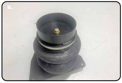
**8.** Bolt the lower bracket to the air spring using a 3/8"-16 x 3/4" hex bolt, 3/8" split lock washer and flat washer. Torque the bolts 15-20 ft-lbs.
