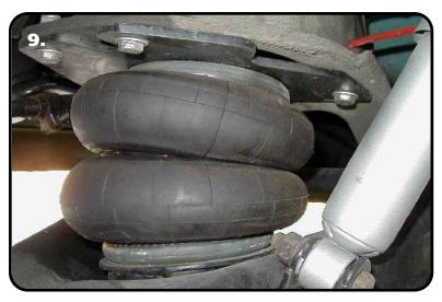
**9.** Attach the air spring assembly to the frame using 3/8" x 1 1/4" bolts, Nylok nuts and flat washers supplied. The lower mount will simply sit in the coil spring pocket. It does not need to be attached. Bolt the frame hardware to 30 ft-lbs.
