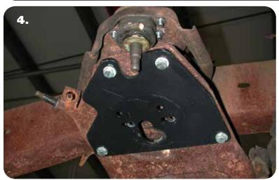
**4.** Hold the upper plate to the cross member as shown in the picture to the left and clamp to frame. Using the plate as a template drill 4 holes in the cross member.
