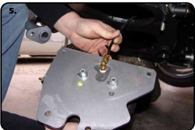
**5.** Apply thread sealant to the air fitting and thread into the air spring. Remove the upper plate from the frame and place onto the studs on the top of the air spring. The holes are lettered; slide the plate to position B moving the air spring to the rear of the vehicle. Secure with 3/8" flat washers and 3/8"-16 nyloc nuts Torque the nuts 15-20 ft-lbs. Route airline.
