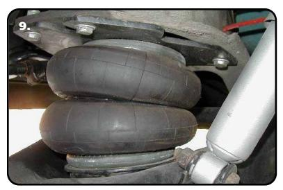
**9.** Attach the air spring assembly to the frame using 3/8" x 1 ¼" bolts, Nylok nuts and flat washers supplied. The lower mount will simply sit in the coil spring pocket. It does not need to be attached. Bolt the frame hardware to 23 ft-lbs.
