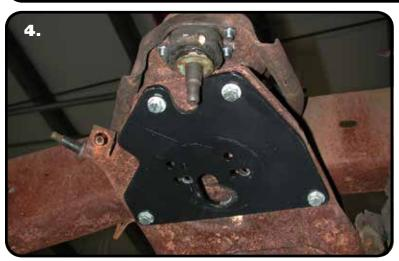
**4.** Hold the upper plate to the cross member as shown in the picture to the left and clamp to frame. Using the plate as a template drill 4 holes in the cross member.
