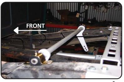
**Note:** This picture illustrates where the MuscleBar is positioned on the frame for drilling the holes. The Swaybar is located in front of the "C"-Notches against the bed support. The arms on the MuscleBar drop down and point to the rear of the truck. On 67-72 Trucks the bed support will aid you in positioning the mounts. On 63-66 the rear tab of the swab bar mount is 5 1/2" from the front of the "C"-Notch (Diagram #2).
