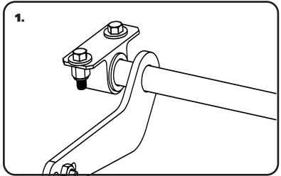
**1.** Install the swaybar bushings and straps onto the MuscleBar. The bushings and straps get installed on the outer ends of the MuscleBar against the stop rings.
