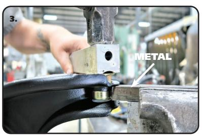
**3.** When installing the 1st Shell, use another Piece of Metal or Strong Wood to Drive the Outer Shell into the Control Arm until the Shell stops against the Control Arm. **Install the Cross Shaft before installing the 2nd Shell.** You will need to use a piece of pipe or a deep socket to install the 2nd Shell due to the shaft sticking through.
