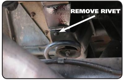
**1.** The Rivet needs to be removed from the rear of the OEM coilspring mount. One way is to cut a "+" in the head of the rivet and chisel the 4 pieces of the head off the rivet, then knock the rivet out of the frame with a hammer and punch. It can also be drilled out.
