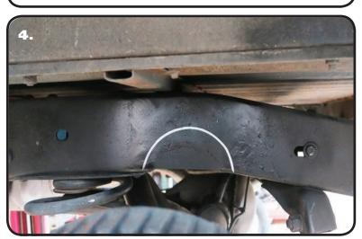
**3.** Use the supplied C-Notch template to mark the area to be cut and the holes to be drilled. We suggest doing one side at a time. The C-Notch template has an arrow pointing to the front of the truck. Use the 5/8" hole to locate the template on the frame. Wrap the bottom tabs around the bottom of the frame. The 2nd Template is provided to aid with the alignment of the bottom holes. The Rivet hole should line up with the front tab. Drill the side holes with a 3/8" drill bit.
