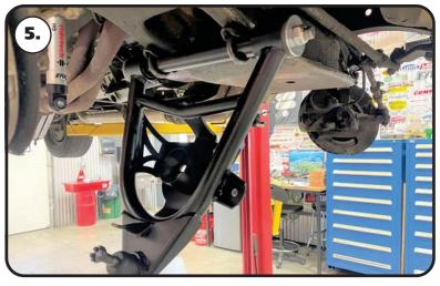
**5. Image 5** is an example of the lower bolted to the crossmember. Install 3/4" ID washer on to each end of the cross shaft against the bushing. Then install the 3/4"-16 lock nut. Snug the nut up against the washer. You want the suspension move freely through its travel.
