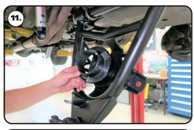
**11.** Place the coil spring isolator over the ring of the control arm.
