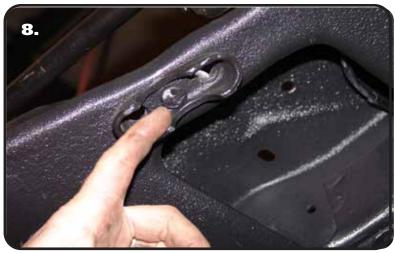
**8.** The lower control arm is installed using the factory u-bolts and nuts. The lower control arm is located by a pin that is in the center of the front u-bolt cradle. This pin will go into the hole in the control arm shaft to help locate the control arm. Bolt the control arm to the frame with the sway bar tab to the front of the truck.
