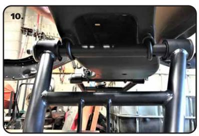
**10. Image 10** is an example of the lower control arm bolted to the crossmember. Install 3/4" ID Washer on to each end of the cross shaft against the bushing. Then install the 3/4"-16 lock nut. Snug the nut up against the washer. You want the suspension to move freely through its travel.
