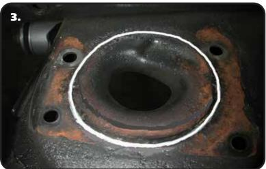
**3.** The top side of the crossmember will also need trimmed for CoilOver clearance. **A TEMPLATE IS PROVIDED ON PAGE 13**. Cut out the holes in the template and place on top of the crossmember. Trace the template onto the crossmember and cut out the center portion. The Template is a guide to the minimum amount that needs to be cut out. Due to variations in the crossmembers, you may need to trim more to get the upper mount to sit flat on top of the crossmember.
