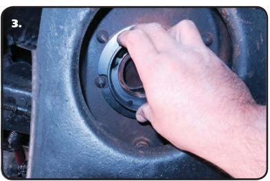
3. The Upper Coil Spring Seat is notched for a Rivet in the OEM Seat. The Notch MUST be lined up with the Rivet when installing the CoilSpring/Seat Combo.
