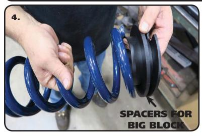
**4.** The CoilSpring Seat is positioned on the top of the Coil Spring with the ring inserted into the CoilSpring. **Small Block requires NO Spacers**. **Big Block trucks require 2 Spacers on the Spring Seat**.
