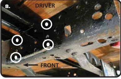
**8.** The rear of the frame has 2 sets of Hanger Mounting Holes, this Kit uses the FRONT set. The Driver side is shown in **Image 8**. Drill the (4) front Hanger mounting holes to 7/16".
