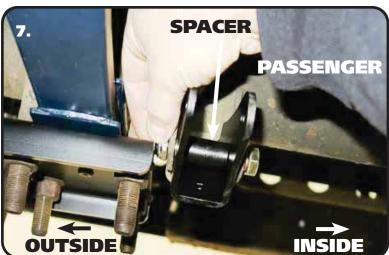
7. The kit includes a spacer that goes inside the New Bracket. Install the 1/2" ID spacer into the Bracket lining it up with the OEM shock holes and holes in the Bracket. Insert a 1/2"-20 x 2 1/2" Bolt through the lined up holes with the THREADS TOWARD THE WHEEL. Install a 1/2"-20 THIN Nylok Nut. Do this for both Shock Mounts. Tighten the 1/2" & 7/16" Hardware on both mounts.
