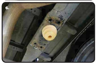
**6.** Install the Bump Stop using a 3/8"-16 x 1" socket head bolt, 3/8" flat washer, & 3/8"-16 nylok nut. Hold the Bump Stop with your hand and insert the bolt through the center of the bump stop. Line up the bolt of the bump with the drilled hole of the frame. Install a 3/8" flat washer and 3/8" nut on the threads of the bolt. Tighten to 120 in-lbs.
