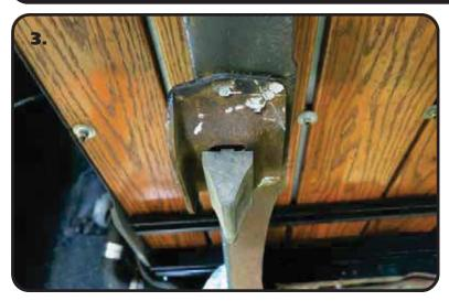
**3.** The OEM bump stop and brackets need to be removed from the frame. Do this by cutting the rivet heads off and driving them out or drilling the rivets out. Remove the driver and passenger brackets.
