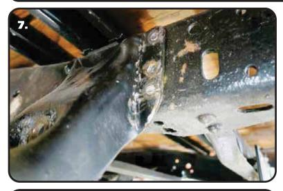
7. The rear leaf spring hanger will need to removed from the frame and replaced with the one included in the StreetGrip Kit. This can be done by cutting a "+"in the head of the rivet and chiseling it off. With the head removed, you can drive the rivet out. The rivets can also be drilled out.
