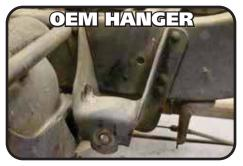
**NOTE:** THIS KIT IS DESIGNED TO BE USED WITH THE OEM FRONT LEAF SPRING HANGER. THE OEM HANGER IS STAMPED STEEL.
