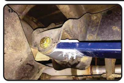
**13.** Swing the front of the Leaf Spring up into the front Hanger aligning the Differential with the Flip Bracket. It may be necessary to raise the Differential up to get the Leaf Spring into the front hanger. Align the holes in the Hanger with the Bushing Sleeve. Install a 9/16" Flat Washer on a 9/16"-12 x 4 1/2" Bolt supplied in this kit. Insert the Bolt/Washer through the Hanger & Leaf Spring. Install a 2nd 9/16" Flat Washer & 9/16"-12 Nylok Nut on the Threads sticking through.
