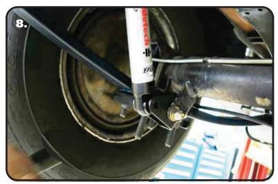
**8.** Slide the bottom of the Shock into the new Mount. Line up the Shock with the Mounting Hole in the Lower Mount. You may need to jack up the differential to get the holes lined up. Install a 1/2" Flat Washer on a 1/2"-20 x 2 1/4" Bolt. Insert the Bolt/Washer into the Mount/Shock. Install a 1/2"-20 THIN Nylok Nut on the threads sticking through. Do this for both sides and tighten hardware.
