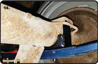
**14.** Lower the Differential down into the Flip Brackets. The Tabs that stick up will rest against the OEM leaf spring mount. This keeps the axle from slipping in the Bracket.
