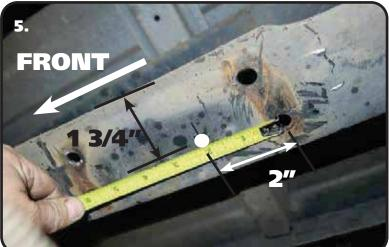
**5.** Once the bump stop mount is removed, a new hole will need to be drilled for the included Bump Stop. Mark the hole 2" from the REAR OUTER rivet hole and 1 3/4" from the INNER Edge of the frame. Mark this location and drill with a 3/8" drill bit.
