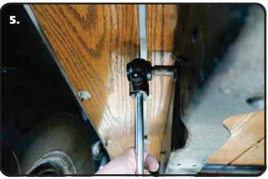
**5.** This Kit includes new upper Shock Studs to replace the existing ones. Replace the Studs and install the eyelet of the Shock on the Stud. The passenger shock gets installed with the Knob forward, install the driver with the Knob to the rear. Once the Shock is installed on the Stud, install a 7/16" Flat Washer & 7/16-20 Nylok Nut on each Stud and tighten.
