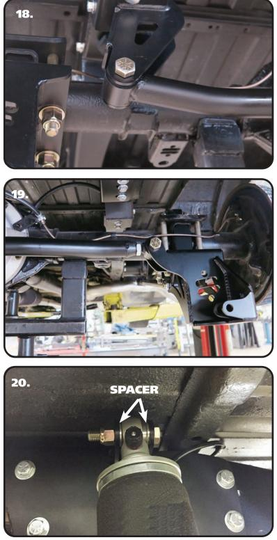
**18.** Install the Panhard bar into the frame bracket. The Panhard Bar is a bent bar, it is bent to clear the center section of the rear differential. The bar needs to be mounted with the BEND to the REAR and the Rubber Bushing in the Frame Mount, this will help it clear the differential cover. The Panhard bar is attached using (1) **5/8" x 3 1/4" bolt**, (1) 5/8" Nylok Jam Nut & (2) 5/8" Flat Washers. Tighten the hardware enough to eliminate any gaps.
