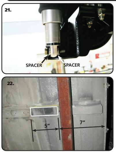
**21.** Insert a Spacer into each side of the lower Shockwave/CoilOver bearing. Slide the shock, with the spacers installed, into the mount on the Lower Axle Mount. You may need to jack the rearend up to line up the holes in the bushings with the 1/2" hole in the shock mounts and hold it in place while you install the 1/2" x 2 1/2" Bolt and 1/2" Nylok Nut with a 1/2" SAE Flat Washer on each side of the mount. Tighten the upper and lower shock bolts to 75 ftlbs.
