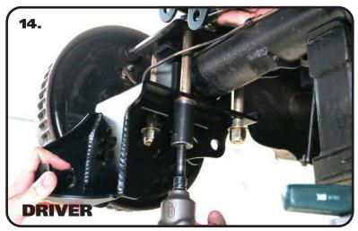
**12.** The Bar Mounts bolt in place of the OEM front leaf spring mount. There is a Driver and Passenger Mount. **Image 12** shows the Driver Mount. The Tabs are to the FRONT of tube. Install a 7/16" Flat Washer on (6) 7/16" x 1 1/4" Bolts. Hold the Mount in place and insert the bolts/washer through the mount and frame. Install a 7/16" Flat Washer and 7/16" Nylok Nut on each bolt sticking through the frame and tighten to 50 ftlbs. Repeat on the other side.
