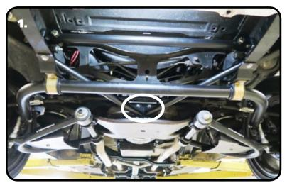
1. Image 1 shows the Frame brace installed. It locates off the bumper & steering box bolts on the drivers side. The passenger side locates off the bumper bolts only. It does require some drilling with a 7/16" drill bit. The rear mounts go up against the crossmember and will need to be drilled too. The area circled in Image 1 is where the braces contact the crossmember.
