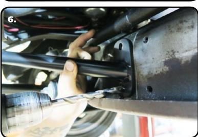
6. Use the Bracket as a template to drill the (4) holes in the crossmember with a 7/16" Drill Bit. Install a 7/16" Flat Washer on each of (4) 7/16"-14 x 1 1/4" bolts and insert them through the bracket and crossmember. Reach through the opening by the lower control arm an insert a 7/16" Flat Washer and 7/16" Nylok Nut on the threads of each bolt. Torque all hardware to 50 ftlbs.
