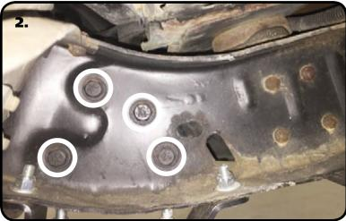
**2.** Start by removing the (2) bumper bolts and (2) steering box bolts on the driver side.
