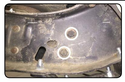
**4.** Remove the bumper bracket bolts from the Passenger side.
