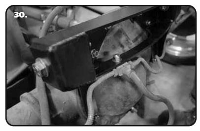
**30.** Using the Hardware Bag "Brake Line Junction Block", install a 5/16" Flat Washer on a 5/16"-18 x 1 1/2" Bolts. Insert the bolt/washer through the junction block and mounting hole in the differential bracket. Install a 5/16" Flat Washer & 5/16"-18 Nylok Nut on the threads of the bolt. The brake lines will need to be tweaked to get the distribution block in position. Torque the bolts to 25 ftlbs.
