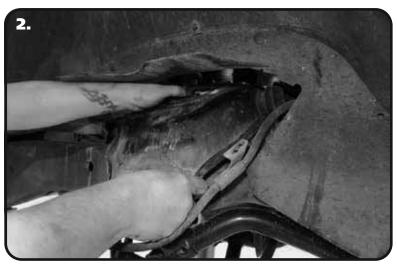
**2.** Remove the Upper Control Arms. The Camber Bolts need to be reinstalled in the same positions they are removed from. We recommend marking their positions for reassembly. Refer to the factory service manual for disassembly procedure. After removing the factory upper control arm, clean the bushing mounting surfaces on the frame.
