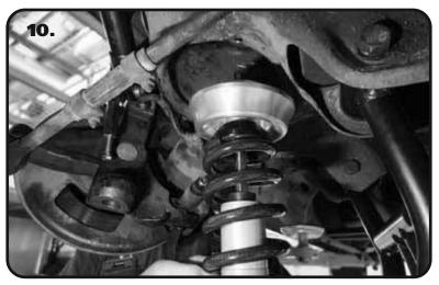
**10.** Insert the CoilOver with the Aluminum Upper installed into the OEM coil spring pocket. You may need to rotate the upper mount while inserting the assembly to get the best alignment of the shock holes.
