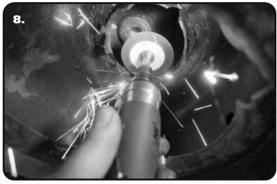
**8.** We used a die-grinder with a cut off wheel to trim the fingers. On some trucks, the holes will line up without trimming
