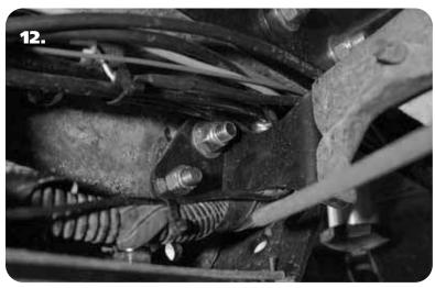
**12.** Slip the Brake Line Bracket over the 7/16" and 5/16" Bolts sticking through the back side of the frame. Install a Flat Washer & Nut on each and tighten.
