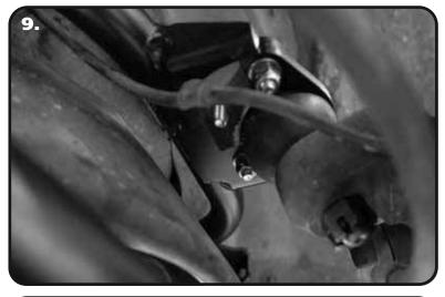
**9.** Attach the ABS cable to the control arm by removing the nut/washer from the front, inner bolt. Slide the bracket onto the bolt and replace the washer & nut. Torque the nut to 25 ftlbs
