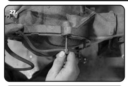
**27.** Thread the Stud into one of the 7 threaded holes in the axle housing. Torque the Stud to 25 ftlbs. Use 2 wrenches to unlock the nuts from each other and remove them from the stud. Repeat the process on the remaining 6 studs.
