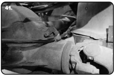
**41.** Slip the mount back in position on the snout of the differential. Reattach it with the OEM hardware that was removed previously. Push the cable down as far as it will go before tightening the hardware. With it in position, tighten the hardware.
