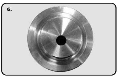
**6.** The Aluminum Upper CoilOver Support has the center mounting hole offset as is the shock mounting hole in the frame. They will need to be test fitted in each side to check for alignment of the OEM shock hole and the shock hole in the aluminum upper mount. It may be necessary to trim the coil spring retaining fingers to get proper alignment.
