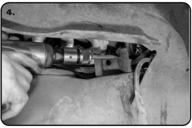
**4.** They make a tool for removing the locating slugs or you can knock them out with an air chisel. It is best to use a blunt tool in the air chisel to knock them out. If you are having a shop align your truck, they will have the tool needed to knock the slugs out.
