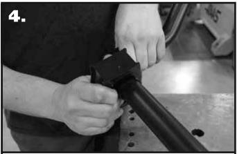
**4.** Open the sway bar bushing at the split and slide it **OVER** the swasy bar. Do this for both bushings.
