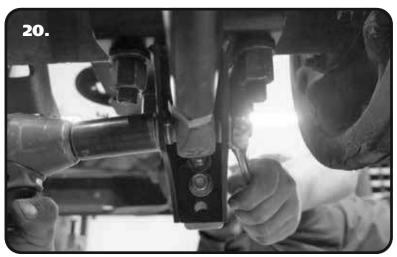
**20.** Install a 5/8" Flat Washer on to a 5/8"-18 x 3" Hex Bolt, insert into the lined up holes. Install a 5/8" Flat Washer followed by a 5/8"-18 Thin Jam Nylok Nut. Repeat on both sides and tighten the Bolts/Nuts enough to eliminate any gaps.
