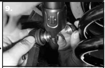
**9.** Insert the 90 degree end link/t-bushing into the swaybar end with the threads pointing toward the coilspring. Install a 2nd t-bushing with the small diameter into the swaybar. Install the nut and torque. Do this for both sides.
