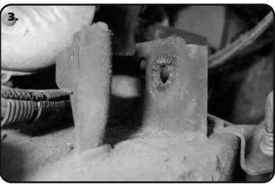
**3.** If your truck has never needed the caster or camber changed, it may still have the locating slugs in the upper control arm mounts. **See Image 3.** Skip to Step 6 if your truck has already had the locating slugs removed.
