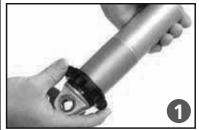
First, using the supplied lower adjuster nut (803-00-199) thread the nut onto the shock from the bottom side as seen in figure 1. Remove the plastic pellet that is in the split of the adjuster nut.
