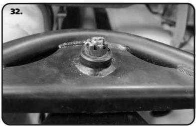
**32.** Torque the ball joint nut to 50 ftlbs. Verify if the hole in the ball joint pin aligns with any of the slots of the castle nut. Tighten the castle nut to align them. DO NOT LOOSEN THE CASTLE NUT. Install the supplied cotter pin. Thread the grease zerk into the ball joint and grease it.
