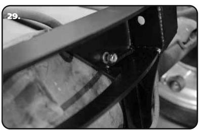
**29.** Using the Hardware Bag "Upper Wishbone Differential Mount", install a M8 Flat Washer & M8-1.25 Nylok Nut on each of (9) M8 Studs. Torque to 225 inlbs
