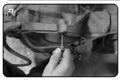
**27.** Thread the Stud into one of the 9 threaded holes in the axle housing. Torque the Stud to 169 inlbs. Use 2 wrenches to unlock the nuts from each other and remove them from the stud. Repeat the process on the remaining 8 studs.
