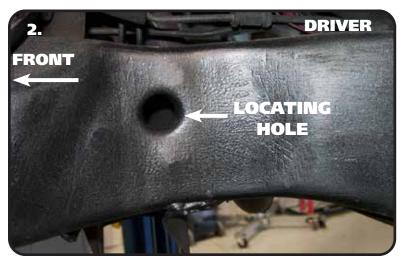
2. Use Images 2 & 3 for installation of the Shock Brackets. DRIVER SIDE IS SHOWN IN THE IMAGES. The Shock Brackets locate off the bottom of the frame rail and the LARGE HOLE that is located to the rear of the coil spring pocket.
