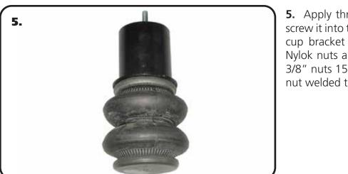
**5.** Apply thread sealant to the air fitting and screw it into the air spring. Assemble the upper cup bracket to the air spring, using 3/8"-16 Nylok nuts and 3/8" flat washers. Torque the 3/8" nuts 15-20 ftlbs. Thread the 8" stud into nut welded to the bottom of the cup bracket.
