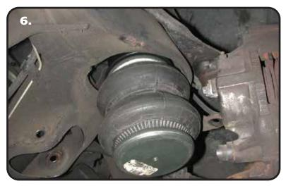
**6.** Place the assembly up into the upper coil spring pocket; the stud will go though the factory shock hole. Fasten with a 7/16"-14 Nylok nut and 7/16" flat washer. Tighten the nut enough to hold the airspring/cup solidly in place.
