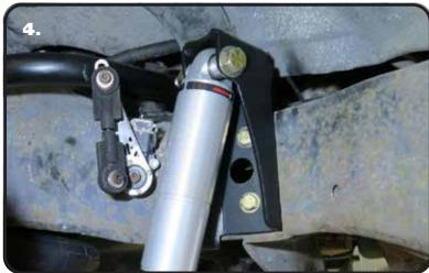
**4.** Insert the SHOCK BODY end of the shock into the shock bracket. Align the through hole with the 1/2" holes in the shock bracket. Install a 1/2" flat washer on a 1/2"-13 x 3 1/2" hex bolt. Insert the bolt/washer through the aligned holes. Install a 1/2" flat washer & 1/2"-13 nylok nut on the threads that are sticking through the bracket. Torque the bolt/nut to 75 ftlbs.
