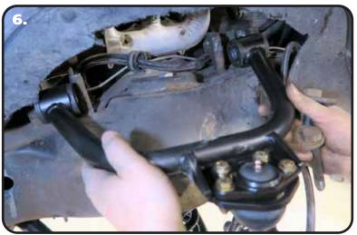
6. Insert the control arm into the OEM location. The Brake Line Tab is positioned to the front of the vehicle. Use the Illustration on page 2 to help aid in installing the correct control arm in the correct location.
