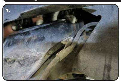
**1.** The OEM upper control arms will need to be removed from the truck. Start by disconnecting the brake line from the upper control arm. Disconnect the ABS cable from the control arm. You will need to remove one of the ball joint bolts to disconnect it.
