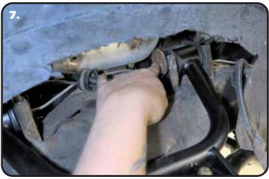
**7.** Bolt the arm to the frame using the factory camber bolts. If you marked the bolts during disassembly, reinstall them in the correct position and tighten. Torque to 140 ft-lbs.
