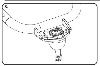
**5.** Install the Ball Joint using the supplied 5/16" Hardware. Insert the ball joint into the arm using **Image 5** as a reference. Insert a 5/16"-18 x 1 1/4" Bolt therough the ball joint and plate. The threads should pointing the same direction as the ball joint pin. Install a 5/16" Flat Washer and 5/16"-18 Nylok Nut on the threads of each bolt. Torque to 18 ftlbs.
