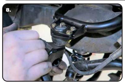
**8.** Slide the ball Joint pin into the spindle and install the castle nut on each one. Torque the ball Joint nuts and install cotter pins in each one.
