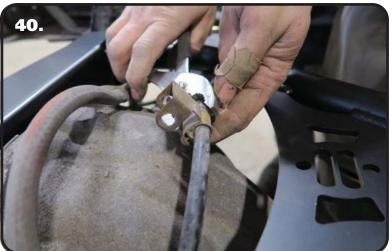
**40.** Use a flat bladed screwdriver to remove the mount from the emergency brake cable. Flip it around so that the bolt hole os to the rear of the truck. Use a pliers to snap the mount back onto the cable.
