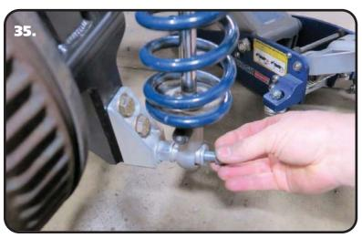
**35.** Install the 7/16" Flat washer and 7/16" Nylok nut. Tighten the upper and lower shock bolts. Torque the Upper Bolt to 50 ftlbs and the Lower Nut to 40 ftlbs. The designed ride height of the CoilOver/Shockwave is 14 1/2" center to center.
