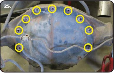
**25.** Remove the top (9) bolts of the differential cover leaving in the bottom (3). The emergency cable will NOT be reattached to the top bolt of the axle. It will get relocated later.
