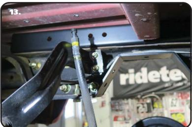
**13.** Install a 5/16" Flat Washer on each of (2) 5/16" x 1 1/4" Bolts. Install the bolts/washers in the Brake Line Bracket and slip the OEM brake line bracket over the (2) bolts. Install a 5/16" Flat washer & 5/16" Nylok Nut on each bolt and tighten.
