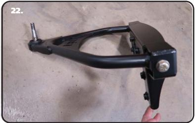
22. Insert the rear of the Wishbone into the Axle Bracket lining up the holes. The ball joint pin needs to be pointing UP. Use **Images 22** & 23 to assist you with positioning of the ball joint pin. Install a 1/2" Flat Washer on each of (2) 1/2"-13 x 3 1/4" Bolts. Insert them into each Bracket/Bushing hole from the outside with the threads pointing to the center. Install a 1/2" Flat Washer and 1/2"-13 Nylok Nut on the threads of each bolt and tighten to 50 ftlbs.
