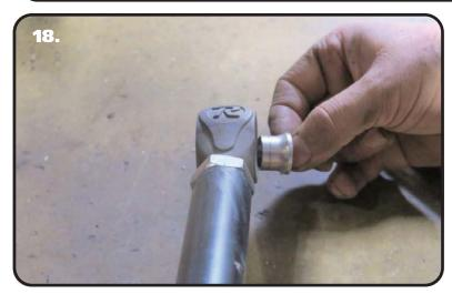
**18.** Insert (2) Narrow R-Joint Spacers into each side of the R-Joint with the small OD inserting into the R-Joint.
