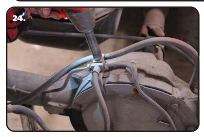
**24.** Remove the bolt that attaches the brake line junction block to the bracket. The junction block will be reattached later.
