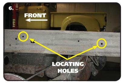
**6.** To allow maximum drop on this truck, the frame must be notched. The template for the notch will locate off of the 2 existing holes. **Image 6** illustrates the holes used. Use the supplied "C" Notch template to mark out the frame for cutting. Before cutting out the frame, support the frame in front of and behind the "C" Notch area. We suggest doing one side at a time.
