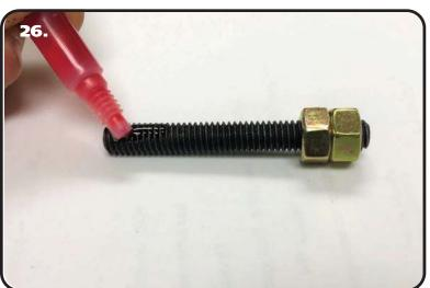
26. The 9 OEM bolts that were removed from the top of the differential cover will be replaced with M8-1.25 x 60mm Studs. These Studs and the nuts used to install them are supplied in the Hardware Bag labeled "Upper Wishbone Differential Mount". Thread the (2) M8-1.25 Hex Nuts on one of the studs. Using (2) wrenches, tighten the nuts against each other locking them together. Apply Red Loctite to the other end of the stud.
