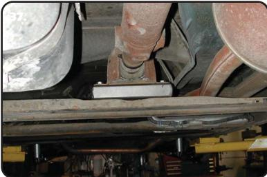
**37.** Install carrier bearing spacer between carrier bearing housing and cross member. Secure with 3/8" x 2 1/2" bolts, 3/8" flat washers, & 3/8" nylok nuts.
