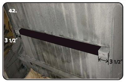
Trimming of the bed brace that is in between the wheel wells is necessary to clear the c-notches and wishbone. We cut ours with a diegrinder and cut off wheel. Image 42 illustrates the bed brace cut out. The cut starts 3 1/2"" from the end of the brace and runs all the way across leaving 3 1/2" on the other end. It needs to be cut even with the flange that attaches the brace to the bed floor.
