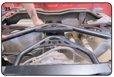
**31.** Install the Rubber Boot on the Ball Joint. **If the rubber boot has a plastic protector on it, discard the plastic protector.** Insert the ball joint pin into the opening of the upper bridge. Push it up in the hole and install the castle nut supplied in the kit.
