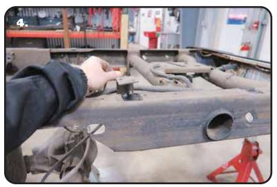
**4.** The brake line bracket will need to be removed from the top of the driver side frame rail. This will be reattached later.
