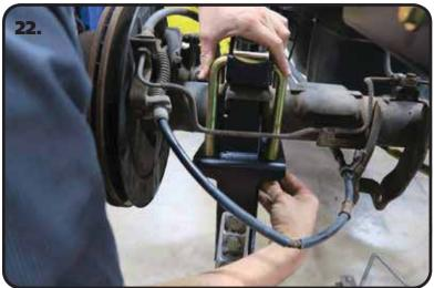
**22.** Hold the mount in place and install a 5/8" flat washer and 5/8" high nut on the threads of the u-bolts sticking through the axle mount. Tighten the nuts evenly in a criss-cross fashion making sure the tabs of the axle mount are touching the leaf spring pad evenly. Torque the nuts in a criss-cross fashion to 60 ftlbs. Repeat on the other side.
