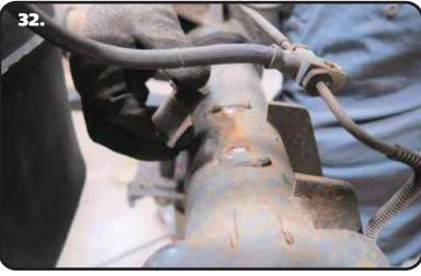
**32.** With both sides of the bracket cut, remove it from the axle tube. Grind the area smooth.
