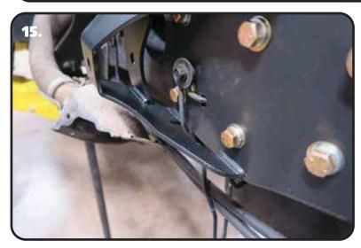
**15.** Reinstall the emergency brake cable bracket using the OEM hardware.
