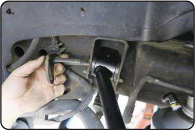
**4.** Bolt the arm to the frame using the factory camber bolts. Torque to 140 ft-lbs.
