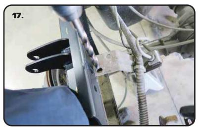
**17.** Use a 7/16" drill bit to drill out the rear hole of the OEM brake line bracket.
