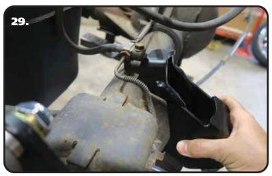
**29.** Depending on the year of your truck, it may have the rear brake hose attached to the axle above the driver side shock mount. If your truck doesn't have the brake line mounted in this location, skip to **Step 33**. If your truck has the brake line mounted in this location, continue to **Step 30**.
