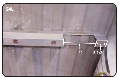
**54.** Trimming of the bed brace that is in between the wheel wells is necessary to clear the c-notches and wishbone. We cut ours with a die-grinder. **Image 54** shows the passenger side, the dimensions are the same for both driver and passenger. The first notch starts 2 1/2" from the end of the brace. The notch is 7" long. Trim the driver and passenger side using these dimensions. **Image 55** shows the driver and passenger sides cut out.
