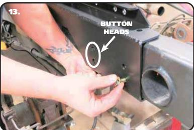
13. Install a 7/16" lock washer, & 7/16" flat washer on (2) 7/16" x 1 1/4" Bolts & (2) 7/16" x 1 1/4" BUTTON HEAD CAP SCREWS. This hardware gets installed in the rear section of the c-notch. THE 7/16" BUTTON HEADS NEED TO BE INSTALL IN THE 2 FRONT HOLES CIRCLED IN IMAGE 13. The 2 regular 7/16" bolts will be installed in the rear holes Install a 7/16" flat washer and 7/16" nylok nut on each bolt sticking through the frame. Repeat on the other side.
