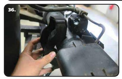
**36.** Position the panhard mount axle clamp on the front side of the axle tube, aligning it with the panhard mount that is already in position.
