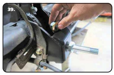
**39.** Insert the short side of the panhard stud into the rear hole of the panhard axle mount. Install a 9/16" SAE flat washer and 9/16"-18 nylok nut on the threads that are sticking through the bracket. Torque to 95 ftlbs.
