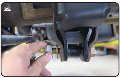
**35.** Install a 9/16" SAE flat washer on a 9/16"-18 x 3 1/2" bolt. Insert the bolt through the OEM lower shock mount and panhard bar bracket. Install a 9/16" flat washer and 9/16"-18 nylok nut on the threads of the bolt. Do not tighten the hardware at this time.
