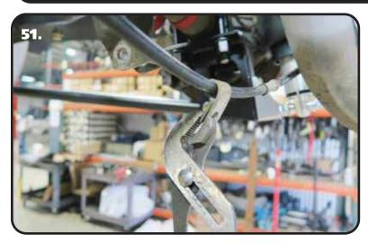
**51.** Reinstall the removed clamp with the ears pointing upward. Install the clamp on the cable and close it with a pair of pliers. Reattach the clamp to the OEM mount using the OEM hardware.
