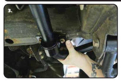
**3.** Slide the MuscleBar into position on the truck. The SwayBar Arms will be above the steering linkage. Install Bushing Straps Over the Poly MuscleBar Bushing and bolt them in place using the OEM hardware. Do not tighten the hardware until the PosiLinks are hooked up to the MuscleBar.
