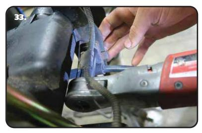
**33.** Unbolt the emergency brake cable clamp from the outside of the driver shock bracket. We will cover reattaching it later in the instructions.
