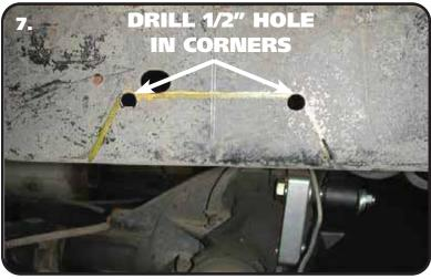
7. Use the supplied Template to mark the cut lines on the frame, then drill out the two corners with a ½" drill bit. This will give the cut a round edge and eliminate the possibility for stress fractures. Then cut the notch with a saw-z-all, cutoff wheel, or plasma cutter. Grind all edges smooth. Check the inside of the frame for wires or lines before drilling or cutting.
