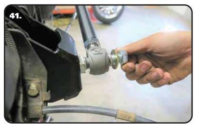
**41.** Install a .625" ID x .740" long R-joint spacer into each side of the R-joint of the axle end of the panhard bar. The small diameter of the spacer goes into the R-joint. Slide the R-joint onto the stud and fasten in place with a 5/8" flat washer and 5/8"-18 THIN nylok nut. Torque to 95 ftlbs.
