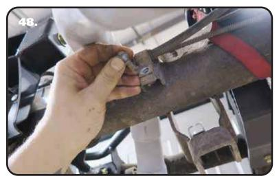
**48. Steps 48-52** cover the emergency brake cable relocation. The cables need to be relocated to gain Shockwave/CoilOver clearance. Start by removing the bolt that clamps the passenger side cable to the driver side axle tube. Spread out the clamp to remove it from the cable. Retain the clamp, it will be reinstalled.
