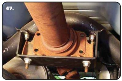
& 3/8"-16 Nylok Nuts. The carrier bearing mount is rotated 180 degrees and attached to the supplied bracket with the OEM hardware as shown in the picture in **Image 47**. The kit includes a Transmission Spacer that will need to be used in conjunction with the carrier bearing mount. Install it by loosening the hardware that attaches the transmission mount to the transmission crossmember. Jack up the rear of the transmission just enough to slide the spacer in and tighten the hardware.
