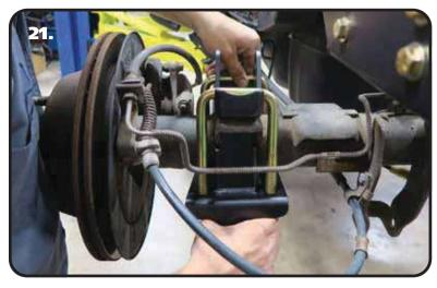
**21.** The axle mounts are the same for driver and passenger sides. Install a supplied 5/8" u-bolt in each side of the upper bar mount. The u-bolts will nest in the slots of the upper mount. Slide an axle mount on the U-bolts with the top tabs inserted into the leaf spring pad.
