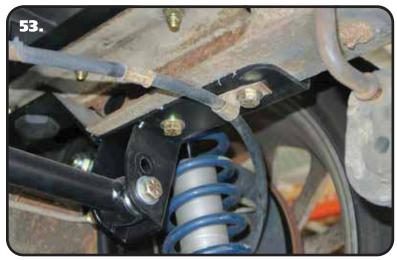
**53.** The passenger emergency brake cable will get attached to the rear bolt of the passenger c-notch. Use the OEM clamp that atthaced it to the axle housing.
