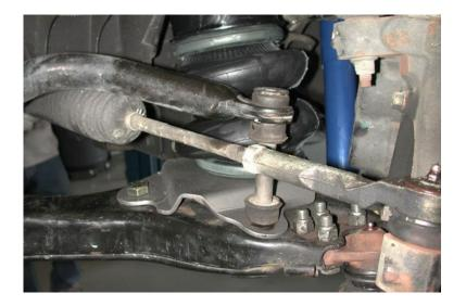
2. Install the lower air spring mounting plate into the lower control arm using the oem sway bar attachment hole as the primary locater. The remaining attachment holes will then be drilled so the plate can be securely fastened to the control arm.
