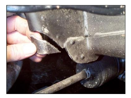
1. The upper coil spring bucket must be trimmed for air spring clearance. The trimmed piece will measure approx. 1  $3/4 \times 1 3/4$ . A die grinder and a cutoff wheel will do the job nicely. The objective here is to create clearance for the air spring. Check this area VERY carefully for abrasion against air spring.
