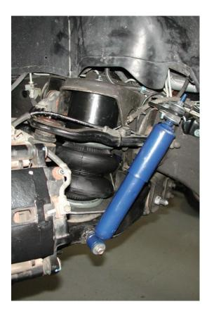
1. The upper shock mount will bolt the rear upper control arm mounting bracket and to the side of the frame rail. It will use one existing hole in the control arm bracket. A  $2^{nd} 3/8$ " hole must be drilled in the control arm bracket. A 5/16" hole must be drilled into the frame rail for the 3/8" self tapping bolts.
