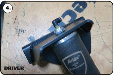
**4.** Put thread sealant on the 90 degree air fittings and thread them into the top of each air spring and tighten.
