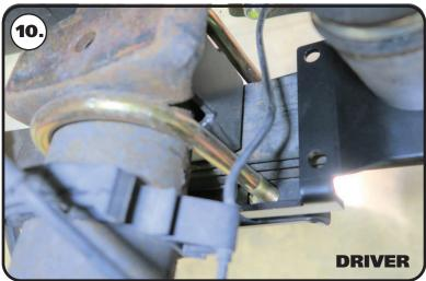
**10.** Use Images 10-13 as a reference for attaching the lower air spring bracket. The bolt holes need to be toward the axle with the forward "hook" hooking the u-bolt. The "hook" will help with positioning of the lower mount. The rear of the mount has 2 tabs that will sit on each side of the leaf spring.
