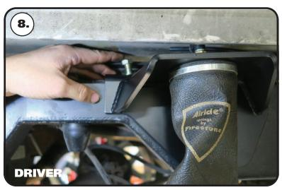
**8.** Install a 7/16" flat washer on each of (2) 7/16" - 14 x 1 1/2" bolts. Insert the bolts/ washers in the 2 top holes.
