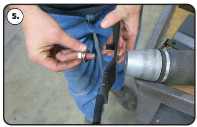
**5.** Attach the lower air spring mount to the bottom of the air spring using a 1/2"-13 x 1" bolt, 1/2" split lock washer, & 1/2" SAE flat washer. DO NOT TIGHTEN AT THIS TIME.
