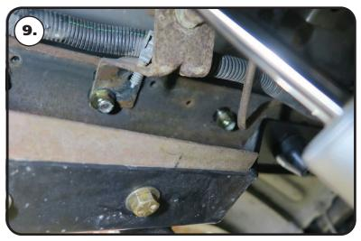
**9.** ON THE DRIVERS SIDE, MAKE SURE THE REAR BOLT IS INSERTED THROUGH THE BRAKE LINE BRACKET. Install a 7/16" flat washer & 7/16"-14 nylok nut on each bolt. Tighten the upper air spring bracket hardware to 50 ft-lbs.
