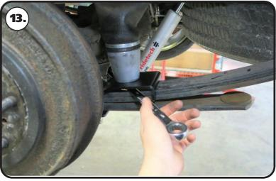
**13.** Tighten the lower 1/2" air spring bolt using a wrench.
