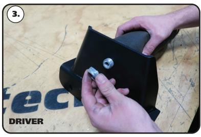
**3.** Thread the 3/4"-16 jam nut on the upper stud of the air spring and tighten with a wrench. DO NOT USE AN IMPACT TO TIGHTEN.
