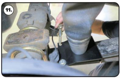
**11.** Install a 7/16" flat washer on each of (2) 7/16" - 14 x 3" bolts. Insert the bolts/washers in the forward 2 holes of the lower bracket.
