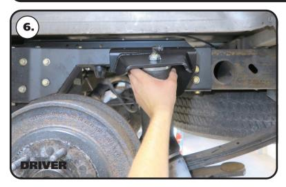
**6.** Insert the air spring/brackets into position. Align the mounting holes with the 4 bolts removed in **Steps 1 & 2**.
