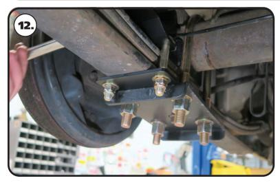
**12.** Slip the spring clamping plate on the threads of the 2 bolts sticking down past the leaf spring. Install a 7/16" flat washer & 7/16"-14 nylok nut on each bolt. Tighten the hardware to 50 ft-lbs.
