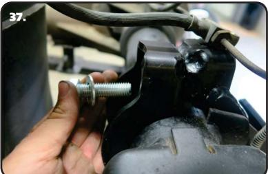
**37.** Install a 1/2" SAE flat washer on each of (2) 1/2"-13 x 1 3/4" bolts. Insert the bolt/washers in the top and bottom mounting holes of the clamp/mount. Install a 1/2" SAE flat washer and 1/2"-13 nylok nut on the threads of each bolt. Torque these bolts to 75 ftlbs. You can now torque the 9/16" hardware that was installed previously. Torque the 9/16" hardware to 110 ftlbs.
