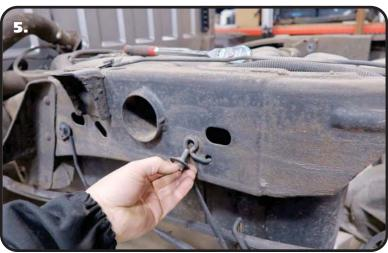
**4.** The brake line bracket will need to be removed from the top of the driver side frame rail. This will be reattached later.
