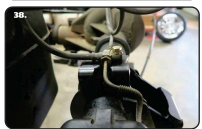
**38.** If your truck required the brake line bracket to be cutoff the axle tube, reattach it to the top of the panhard mount. Use the  $5/16"-24 \times 1"$  bolt, 5/16" split lock washer, & 5/16" SAE flat washer that's supplied in the kit.
