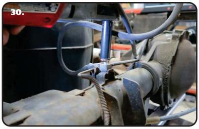
**30.** Remove the bolt that attaches the brake hose to the bracket. This will allow you to move the brake line out of the way to cut the bracket off the axle tube.
