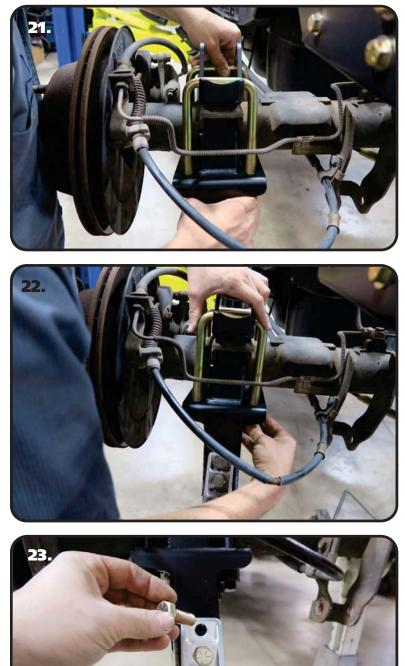
**21.** The axle mounts are the same for driver and passenger sides. Install a supplied 5/8" u-bolt in each side of the upper bar mount. The u-bolts will nest in the slots of the upper mount. Slide an axle mount on the U-bolts with the top tabs inserted into the leaf spring pad.
