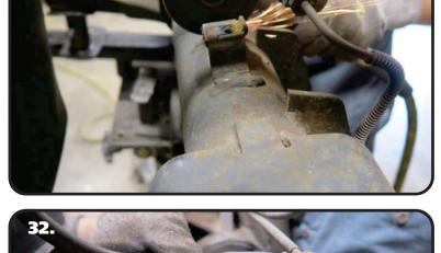
**32.** With both sides of the bracket cut, remove it from the axle tube. Grind the area smooth.
