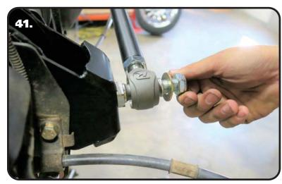
**39.** Insert the short side of the panhard stud into the rear hole of the panhard axle mount. Install a 9/16" SAE flat washer and 9/16"-18 nylok nut on the threads that are sticking through the bracket. Torque to 95 ftlbs.
