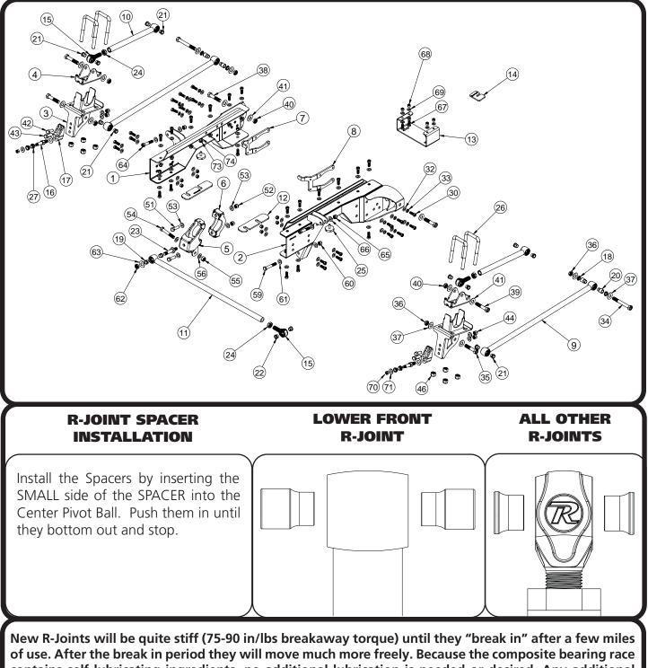
contains self lubricating ingredients, no additional lubrication is needed or desired. Any additional lubrication will only serve to attract more dirt and debris to the R-Joint and actually shorten its life.
