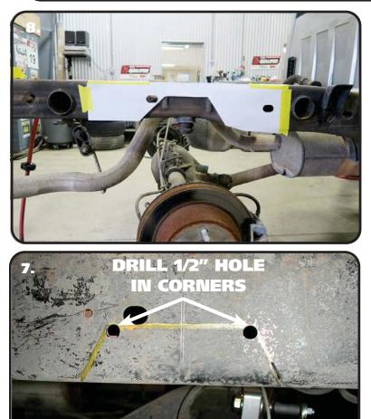
**6.** To allow maximum drop on this truck, the frame must be notched. The template for the notch will locate off of the 2 large oval holes. Use the supplied "C" Notch template to mark out the frame for cutting. Before cutting out the frame, support the frame in front of and behind the "C" Notch area. We suggest doing one side at a time. The tall end of the template is located to the front of the truck.
