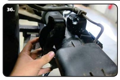
**36.** Position the panhard mount axle clamp on the front side of the axle tube, aligning it with the panhard mount that is already in position.
