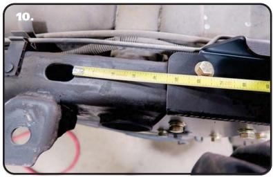
**9.** After cutting, slip the c-notch over the frame to check the fitment.
