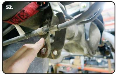
**52.** The Driver side emergency brake cable only requires the clamp be moved on the cable. Remove the attaching bolt and spread out the clamp enough to allow it to be moved. Move the clamp from the metal area to the rear edge of the plastic sheath. The rear edge of the sheath. Use the OEM bolt to reattach it.
