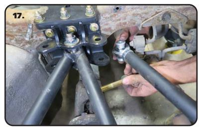
**17.** Insert a WIDE spacer in each side of the rear heim. The small diameter of the spacers will insert into the heim end. Insert the heim/ spacers into the mount on the front wishbone mount. You will need to adjust the bar to get the holes of the mount aligned with the heim/ spacers. The bars are threaded left and right, they will adjust in and out evenly by turning the bar.
