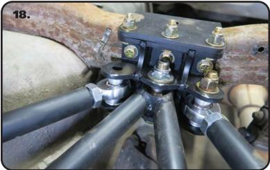
**18.** Adjust the bar to get the through hole of the heim/spacers aligned with the mounting holes of the wishbone mount. Install a 1/2" SAE flat washer on a  $1/2"-13 \times 3 1/4"$  bolt. Align the through hole of the heim/spacers with the holes of the mount. Insert the bolt/washer in the lined up holes. Install a 1/2" SAE flat washer and 1/2"-13 nylok nut on the threads of the bolt.
