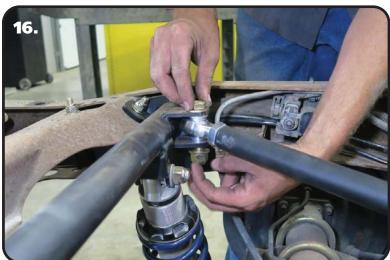
**16.** Install a 1/2" SAE flat washer on a 1/2"-13 x 2 1/2" bolt. Align the through hole of the heim/spacers with the holes of the mount. Insert the bolt/washer in the lined up holes. Install a 1/2" SAE flat washer and 1/2"-13 nylok nut on the threads of the bolt.
