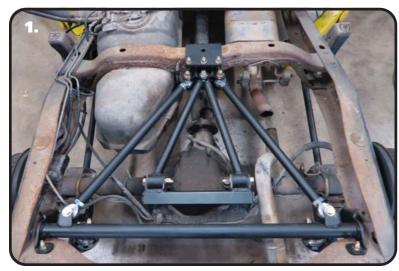
**1. Image 1** shows an overview with the brace bars installed. The wishbone setup in your truck has to have the provisions for the brace bars.
