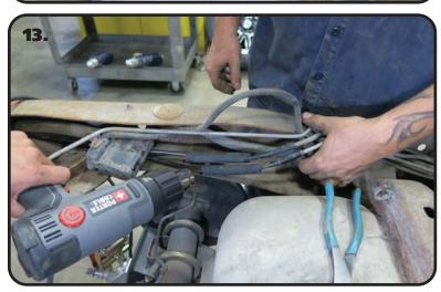
**11.** Cut the supplied plastic line in half. Run the 2 pieces of line through the driver frame rail. It will run from where you cut the lines, back to the canister. Cut the supplied heat shrink into 4 equal pieces. Slide the pieces of heat shrink on each end of the lines you just ran.
