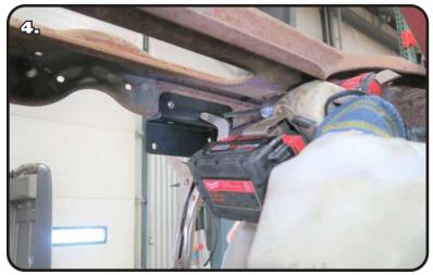
**4.** Drill the (4) mounting holes using a 3/8" drill bit. Use the bracket as a template to drill the holes.
