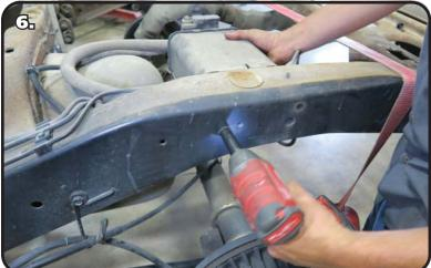
**5.** Install a 3/8" flat washer on each of the (4) 3/8"-16 x 1 1/4" bolts. Insert (1) bolt/washer into each of the drilled holes. Install a 3/8" flat washer and 3/8"-16 nylok nut on each bolt. Torque to 30 ftlbs.
