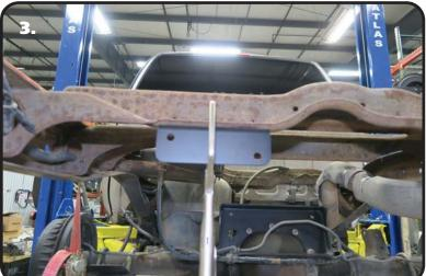
**3. Image 3** illustrates the location of the bracket for relocating the emissions canister. Notice that the staggered holes are the ones that hang down.
