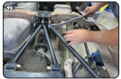
**19.** With the bar installed, tight the jam nuts against the bar.
